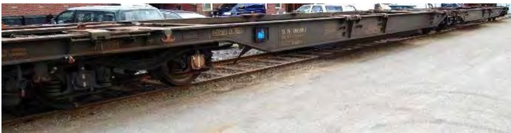
Figure 5: 6-axled container freight car.
