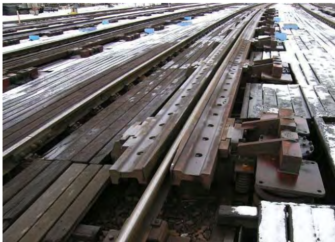
Figure 8: The mechanical brake is a beam brake that pinches against the freight car wheels.
