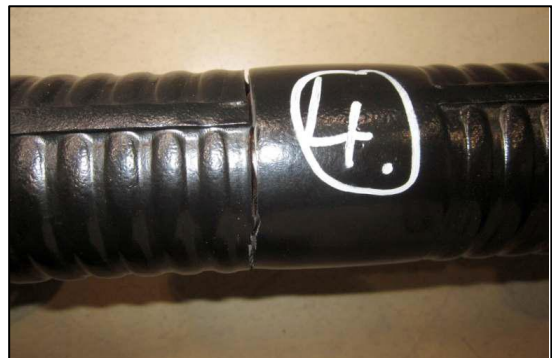
Figure 17: Break in tube during durability test 4 [10].
