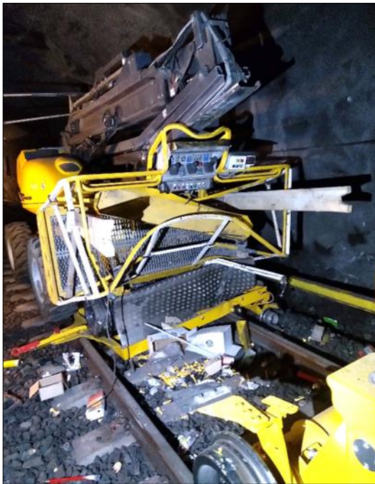
Figure 1: The MEWP after the collision. Photo: BMO Entreprenør AS
