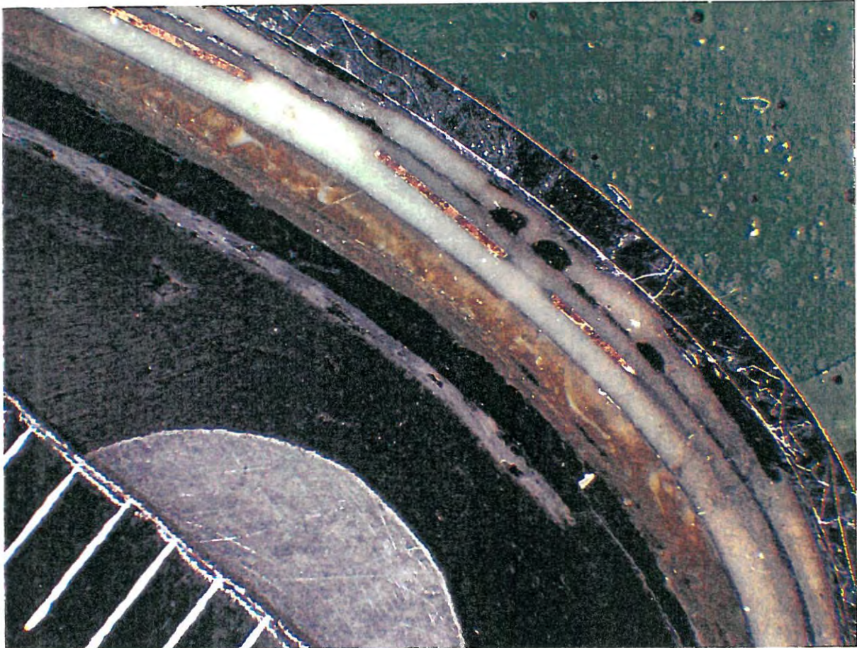
Metallographic close-up photo illustrating the composition/structure of the leading edge section of the main rotor blade.
