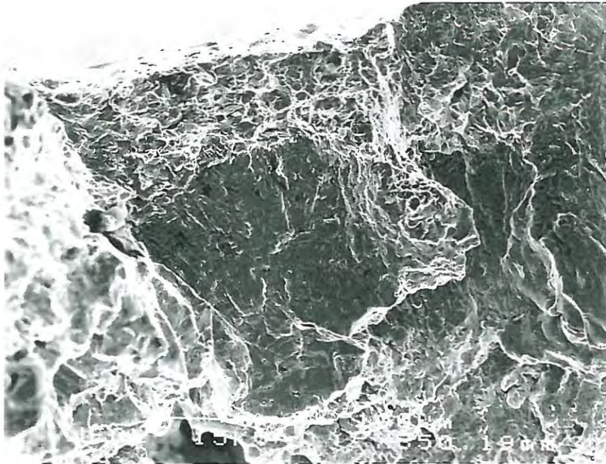
Another smooth fracture surface area in the section S1, detail from the area framed in Fig. 35B.
