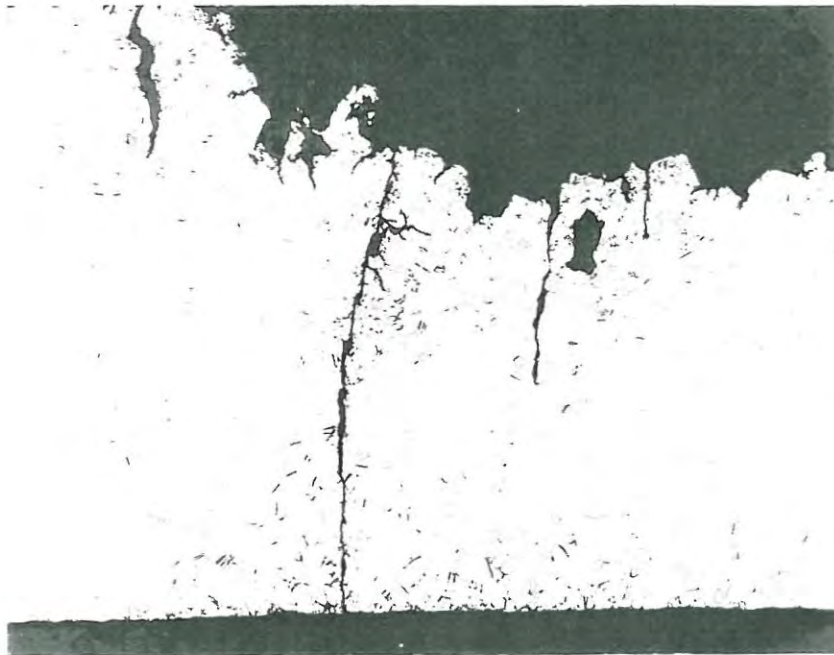
Micrograph illustrating the situation of erosion and cracking within a local transverse section of the protective Ti-strip, leading edge position. Magnification x 160.
