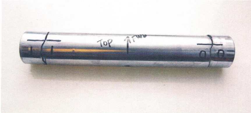
Figure 1 Picture of fractured Fuse-Pin, marked with forward direction (FWD) and inner (I) and outer (O) side. The black line across the two corresponding fracture parts is defined as the 12 o'clock position in the following
