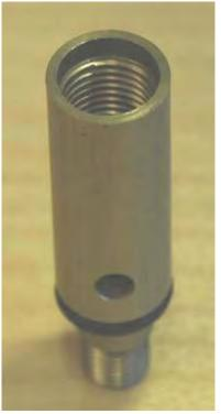
Figure 4: Standpipe (part number 0756036-2) with short thread section (inner threads starting 0.120" from the flange).
