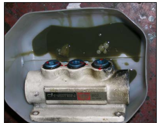
Figure 2: Ice and oil drained from the Christen 802 valve
