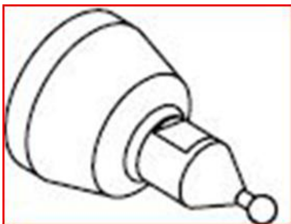
Figur 11-5 Ball point probe (FARO User Manual, 2007)
