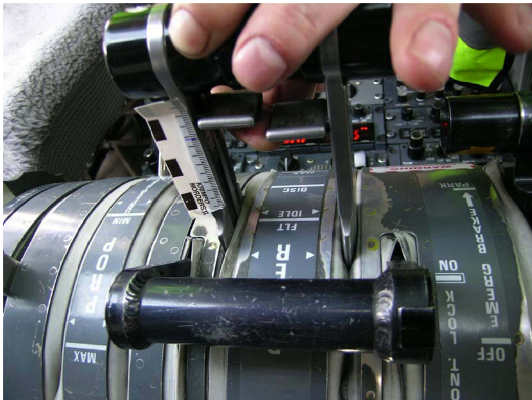
Figure 3: The Power Lever trigger mechanism shown must be lifted by the pilot in order to allow the Power Levers to pass through the FLT IDLE gate while moving aft into the ground Beta-range. The trigger for the right engine (left in picture) has been disengaged. The picture is taken from the instrument panel looking aft. The black lever in front is the flight control lock. The measuring tape is attached by AIBN.
