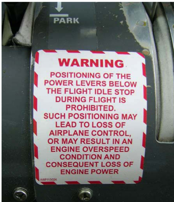
Figure 10: Warning sign installed near the Power Lever.
