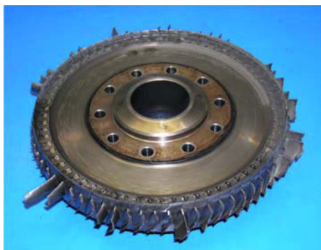
Figure 8: Damage to the power turbine's second stage.
