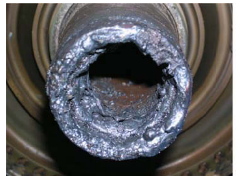
Figure 9: The low pressure turbine shaft had separated and partially melted.
