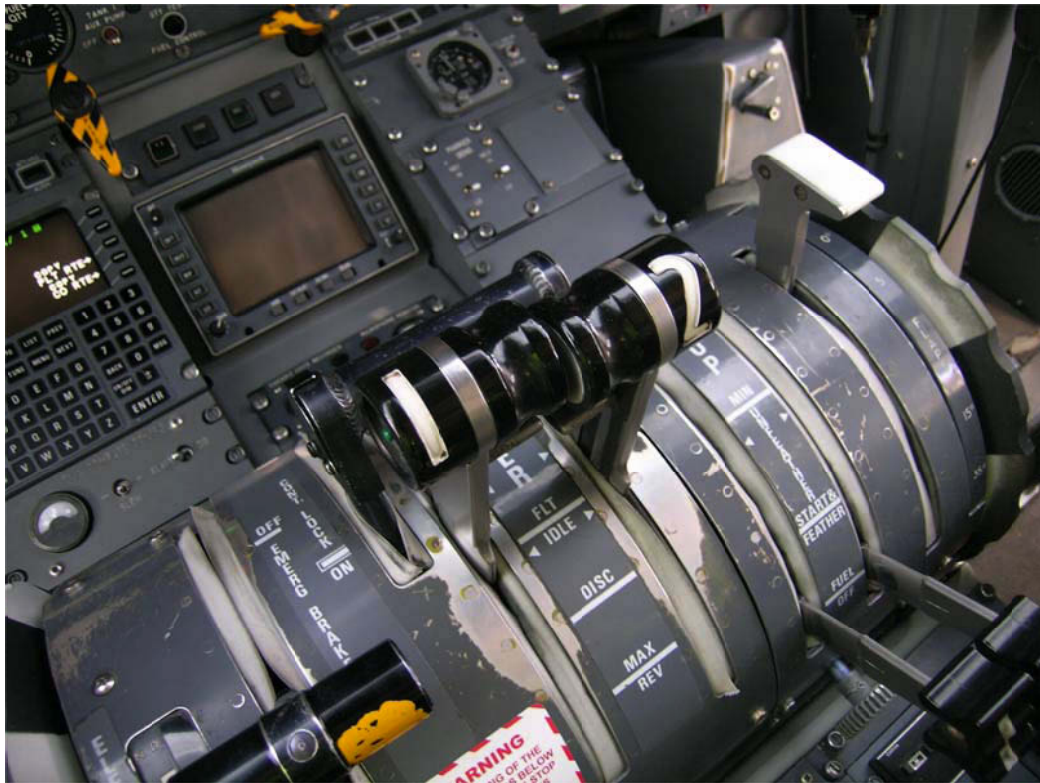
Figure 2: Power Levers marked 1 and 2 in the centre of the photo and condition levers in the bottom right corner (Fuel Off).
