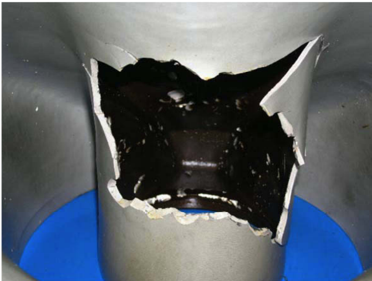
Figure 7: Damage to the air intake on the right engine which arose when the shaft between the engine and gear box separated.
