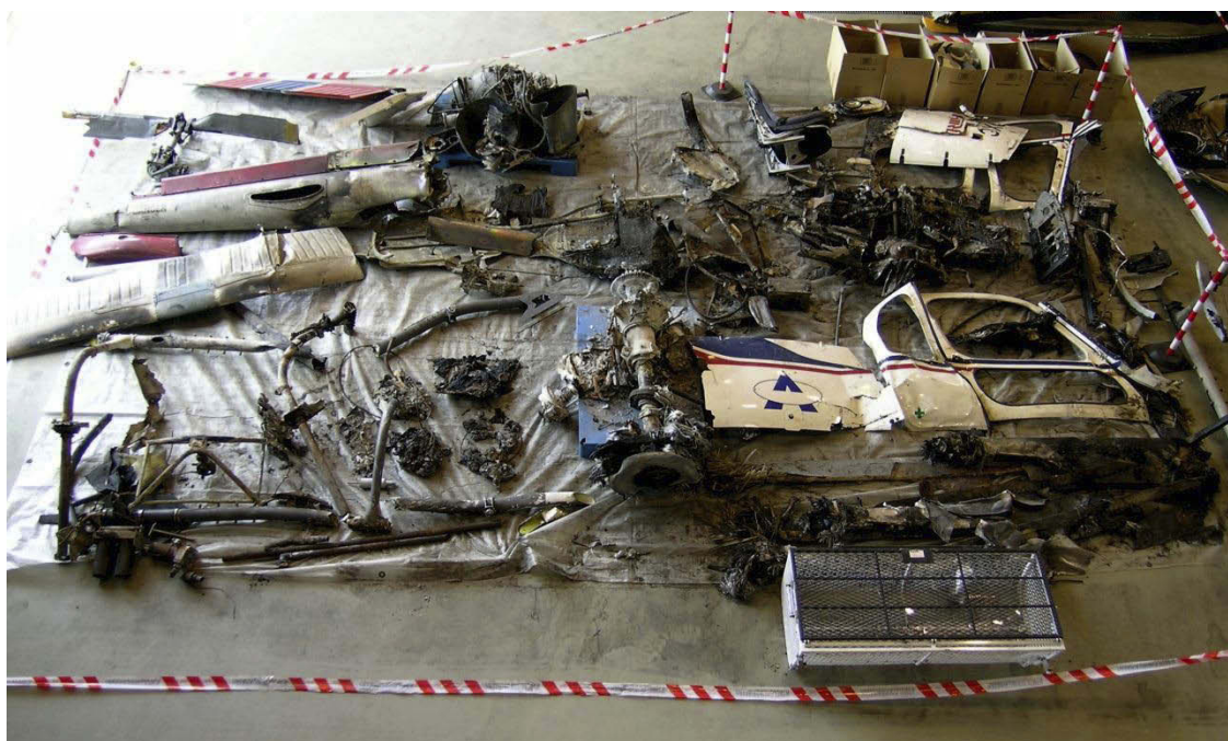
Figure 9: Simplified reconstruction of the wreckage in the Accident Investigation Board's hangar.
