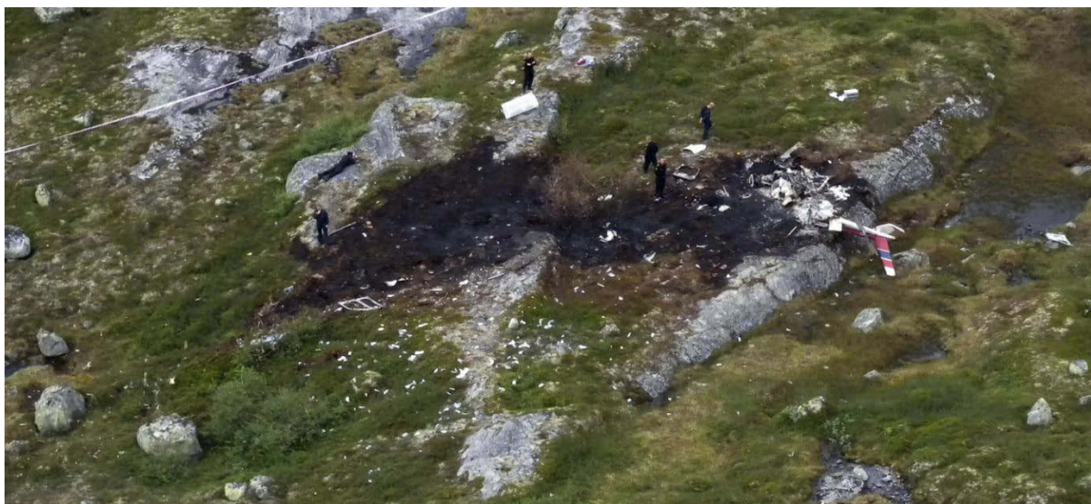
Figure 5: The accident site seen from the east. The helicopter moved from the left to the right in the picture and hit the ground to the far left of the burned area. Cf. also site mapping in Appendix B.
