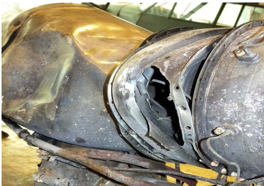
Figure 10: The penetrated containment shield.
