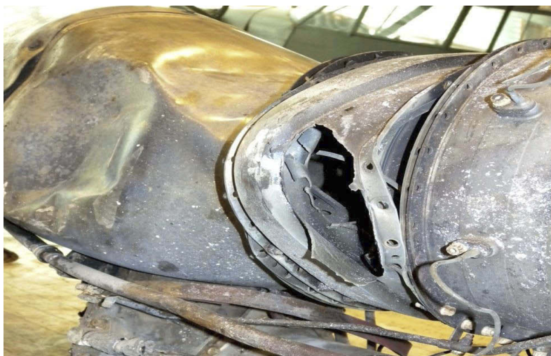
Figur 10: Hullet i Containment shield.
