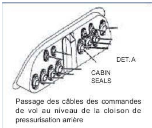
Passage of flight control cables at the aft pressurized bulkhead
