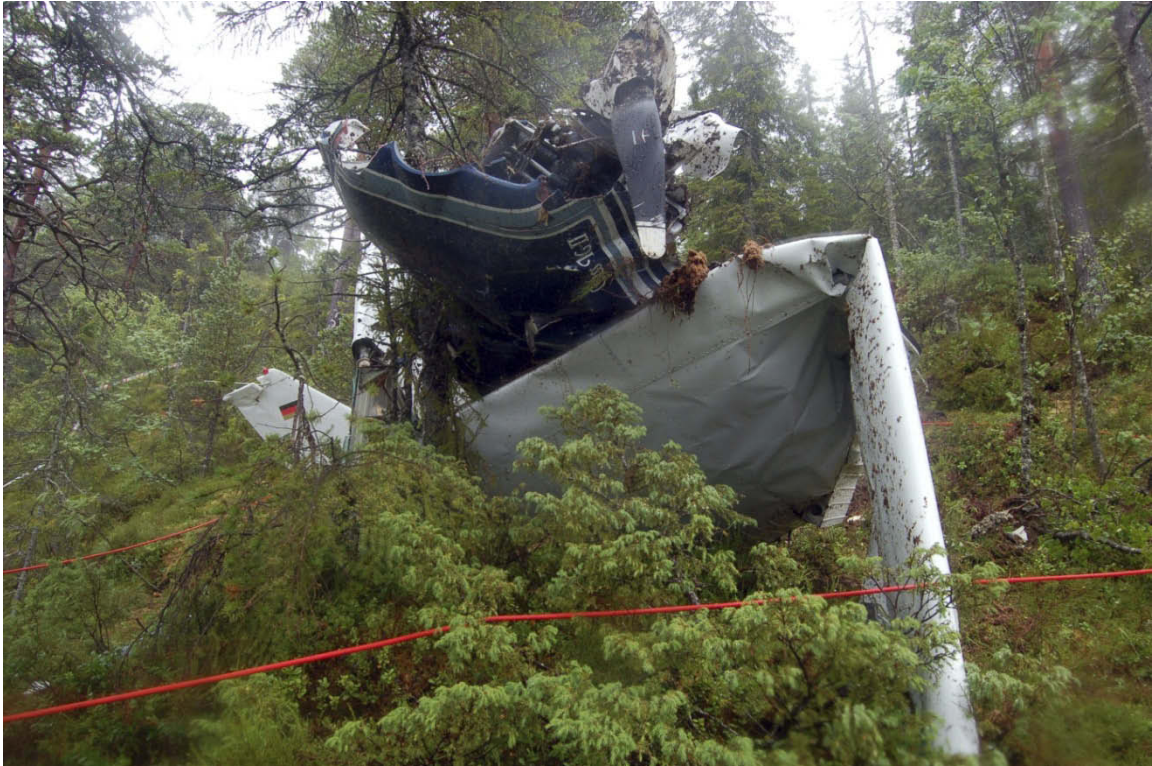
Figure 10: The front of the wreckage. The engine lies on top of the folded-up right wing. (Photo: AIBN)
