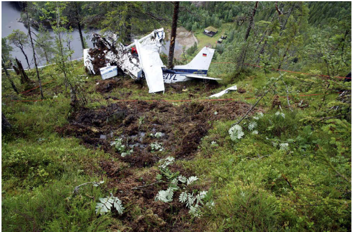
Figure 9: The accident site viewed in a north-easterly direction. The cabin by the lake where the eye witness was located is visible in the background. The groove created by the left wing and the crater left by the engine are visible in front of the wreckage. (Photo: AIBN)
