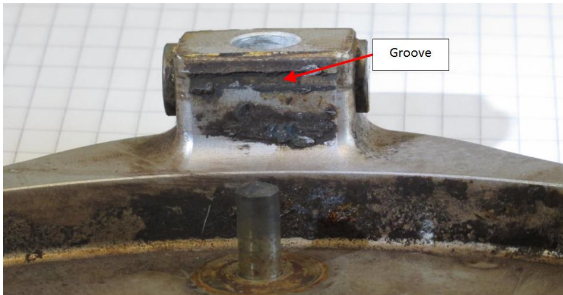
Figure 14: Bracket with wear marks (groove) from the friction disc. Photo: AIBN
