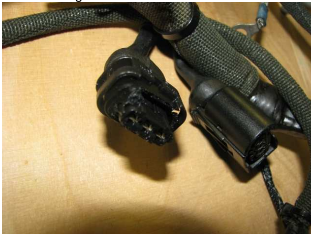
Picture 4 Damage to the connector shell
