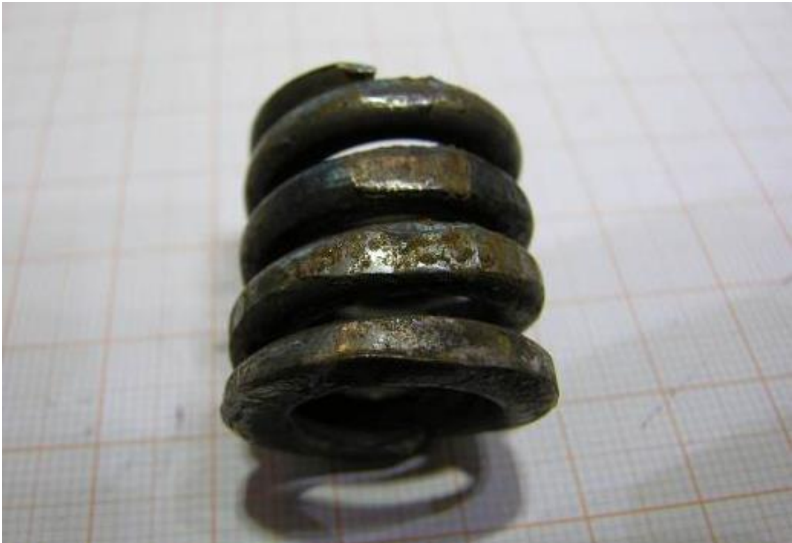
Figure 12: Wear marks on one of the coil springs after scraping against the fracture surfaces in the inner part of the Clutch Hub. Photo: AIBN
