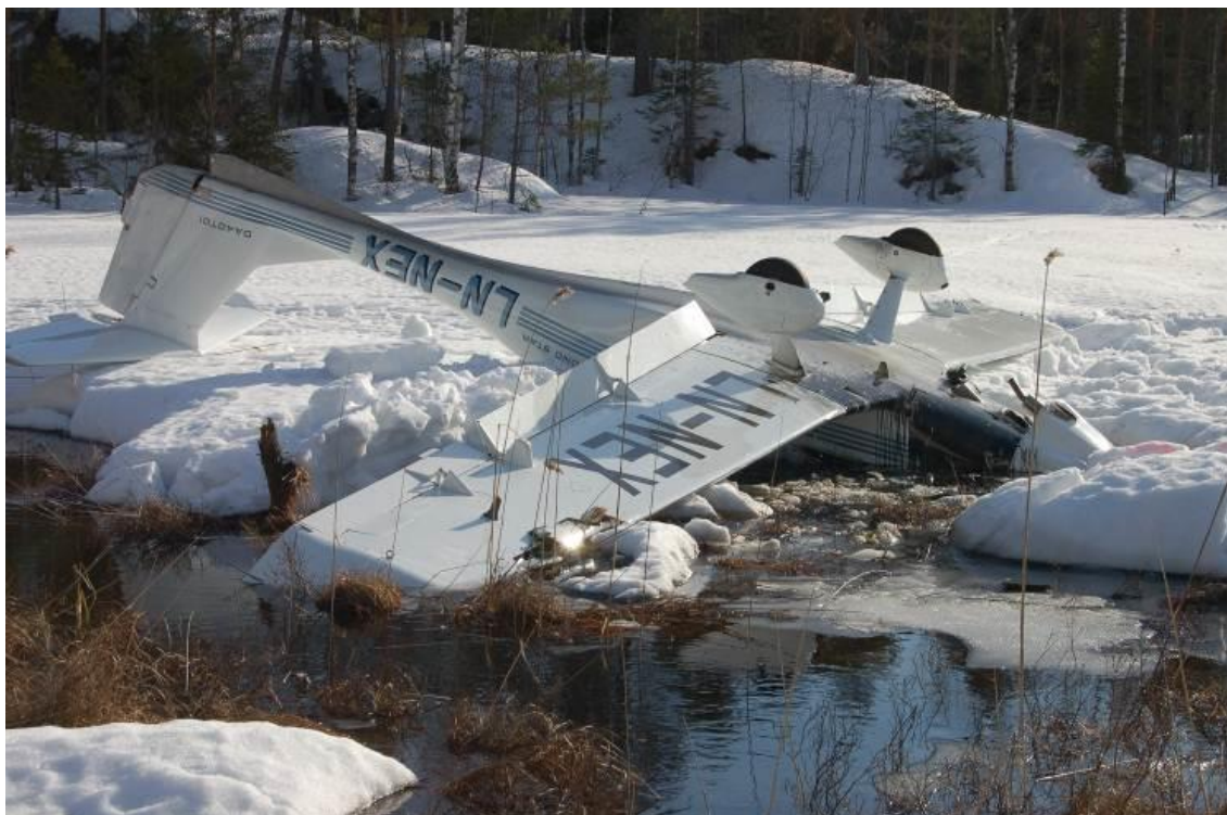
Figure 1: LN-NEX resting upside-down after the forced landing. The photo shows oil spillage on the fuselage behind the engine cowling and on the lower left wing (in front of the L/H main landing gear leg). Photo: AIBN
