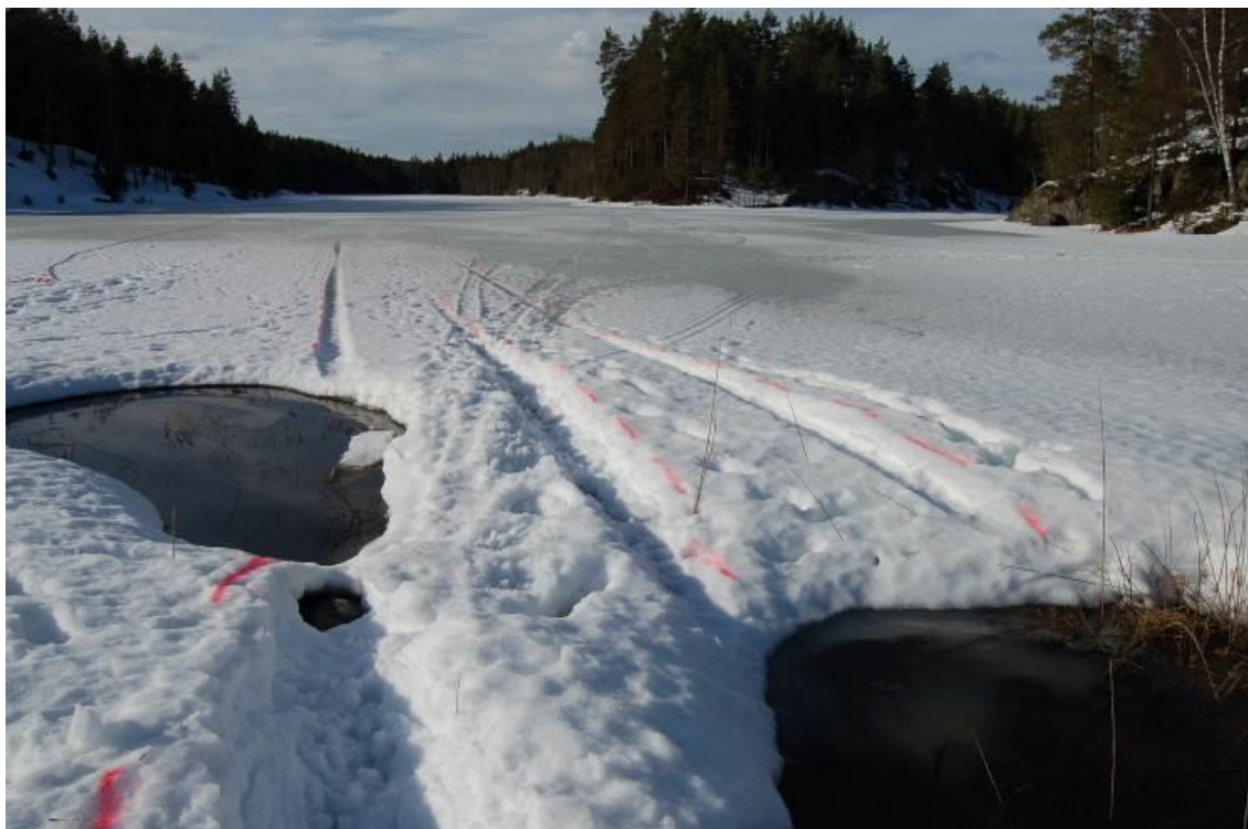
Figure 2: The wheel tracks in the snow (dyed red) seen from where the aircraft stopped. Photo: AIBN
