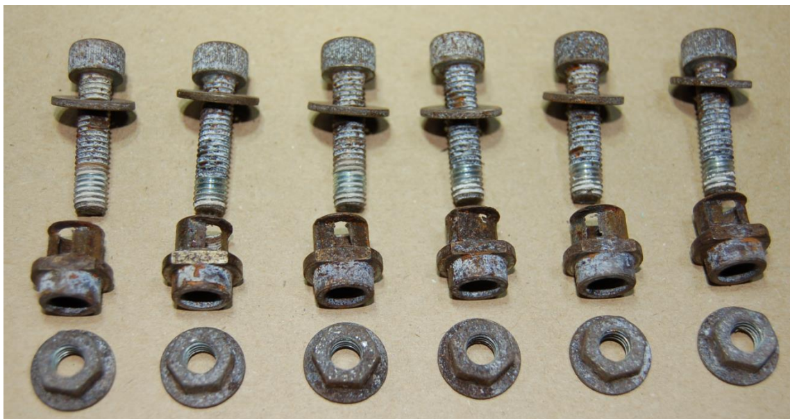
Figure 10: The bolts that hold the Clutch Hub and the adjacent hubs together. Impacts from the Clutch Hub have worn a hole through all the sleeves. Photo: AIBN
