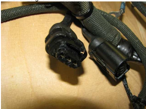
Picture 4 Damage to the connector shell
