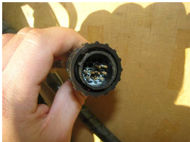
Picture 3 Signs of oxidation
