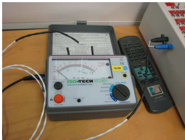
Picture 9 Isolation tester
