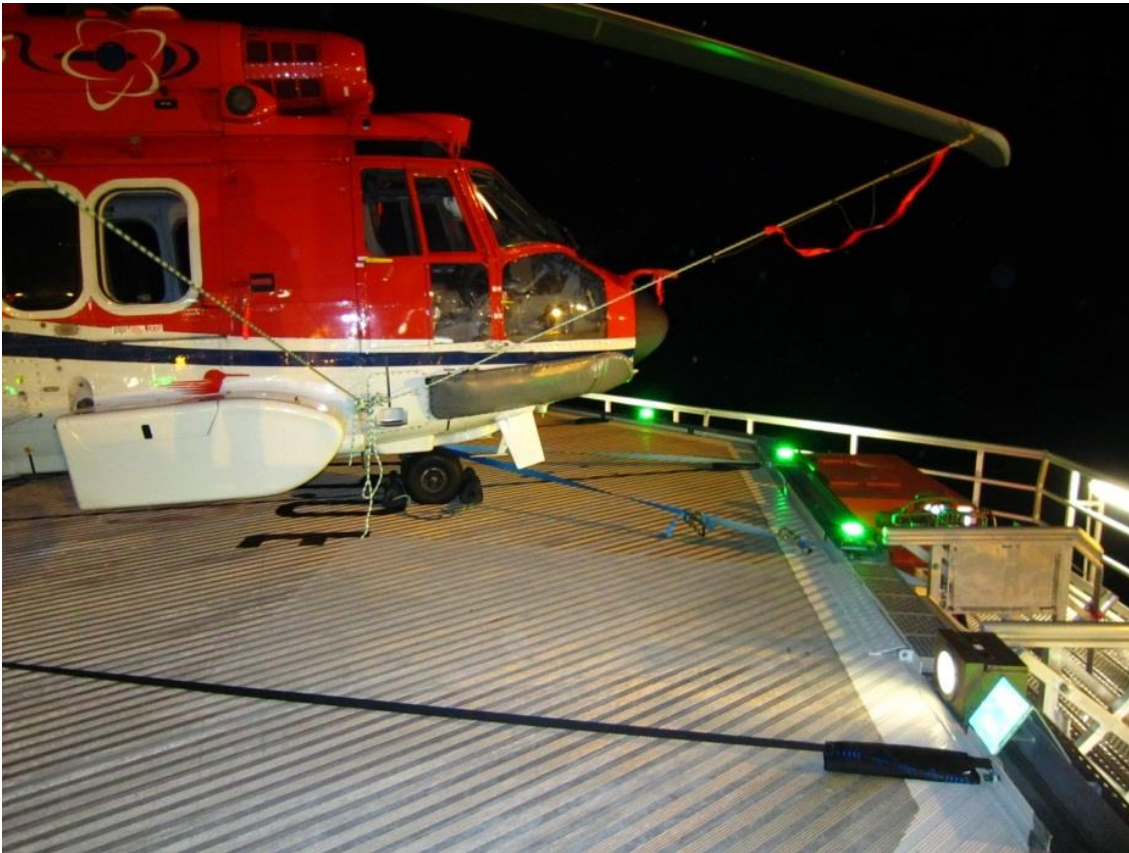
Figure 3: LN-OJE where it stopped on the helicopter deck on Åsgard B after the landing. The picture also shows the edge of the helicopter deck, the gutter and the walkway. Photo: STATOIL
