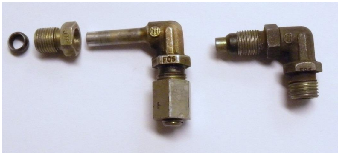
Figure 5: The elbow union from LN-OJE to the left. An elbow union with a correctly installed compression ring to the right. The compression ring (dark) that came loose to the left. Photo: AIBN
