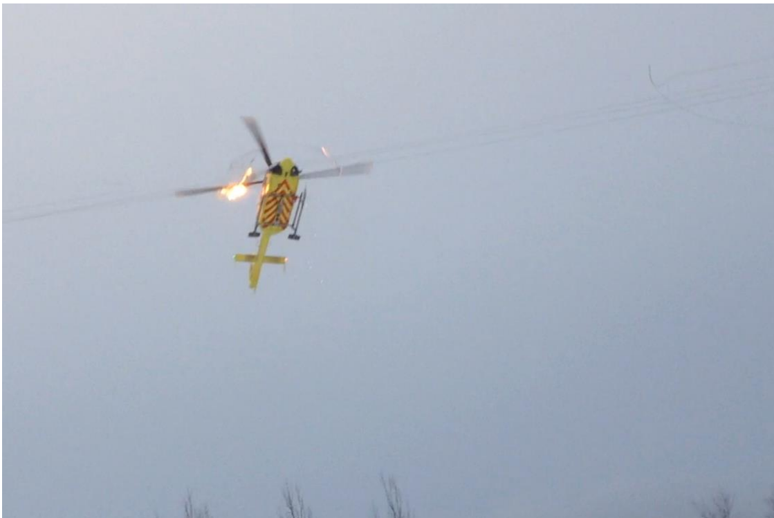
Figure 3: Immediately after the main rotor has cut one of the live lines. One of the ends of the line is moving out of the image towards the right. Another section of the line is about to be slung by the rotor. Photo: Still image from a private video recording
