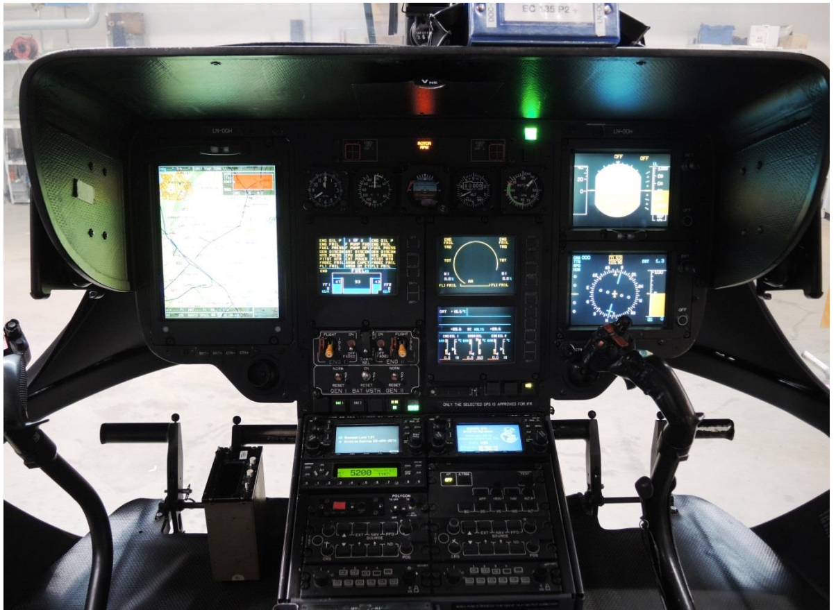
Figure 7: Cockpit in one of the Air Ambulance's EC 135s. The large display on the left is operated by the HEMS crew member. He can choose to view the moving map on the entire display, as shown in the picture, or to split the display, as shown for the pilot on the right. A third possibility is that the display on the left shows flight instruments on the top half and the moving map on the lower half of the display (see Figure 8). Photo: AIBN
