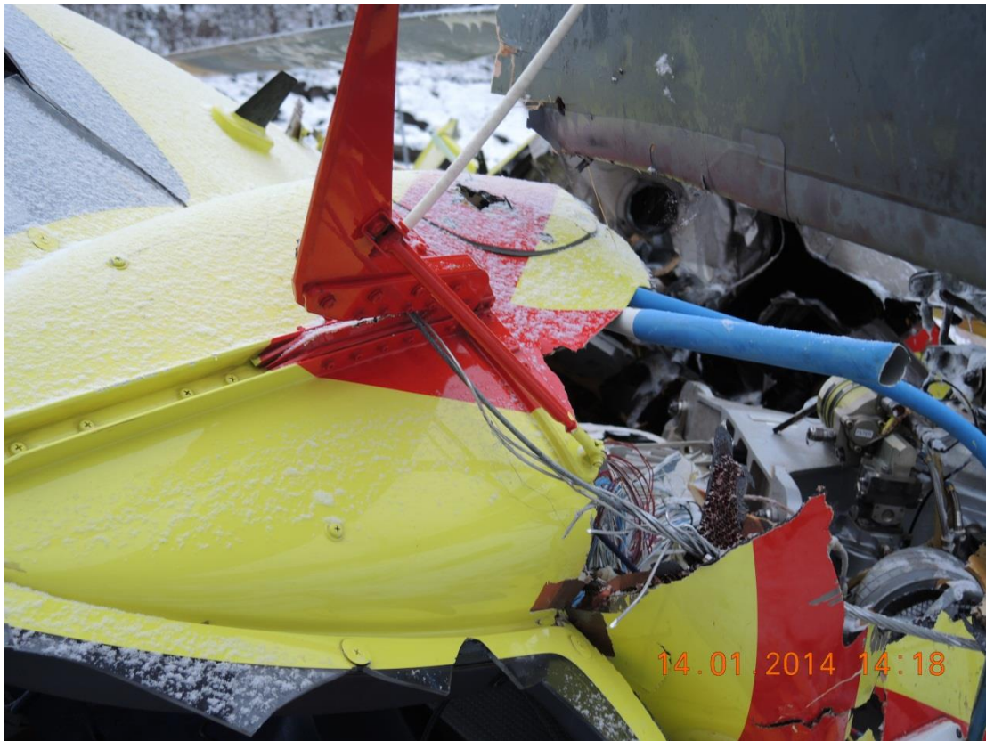
Figure 5: One of the lines from the power line stuck in the wire cutter on the cockpit roof on LN-OOI. Photo: AIBN
