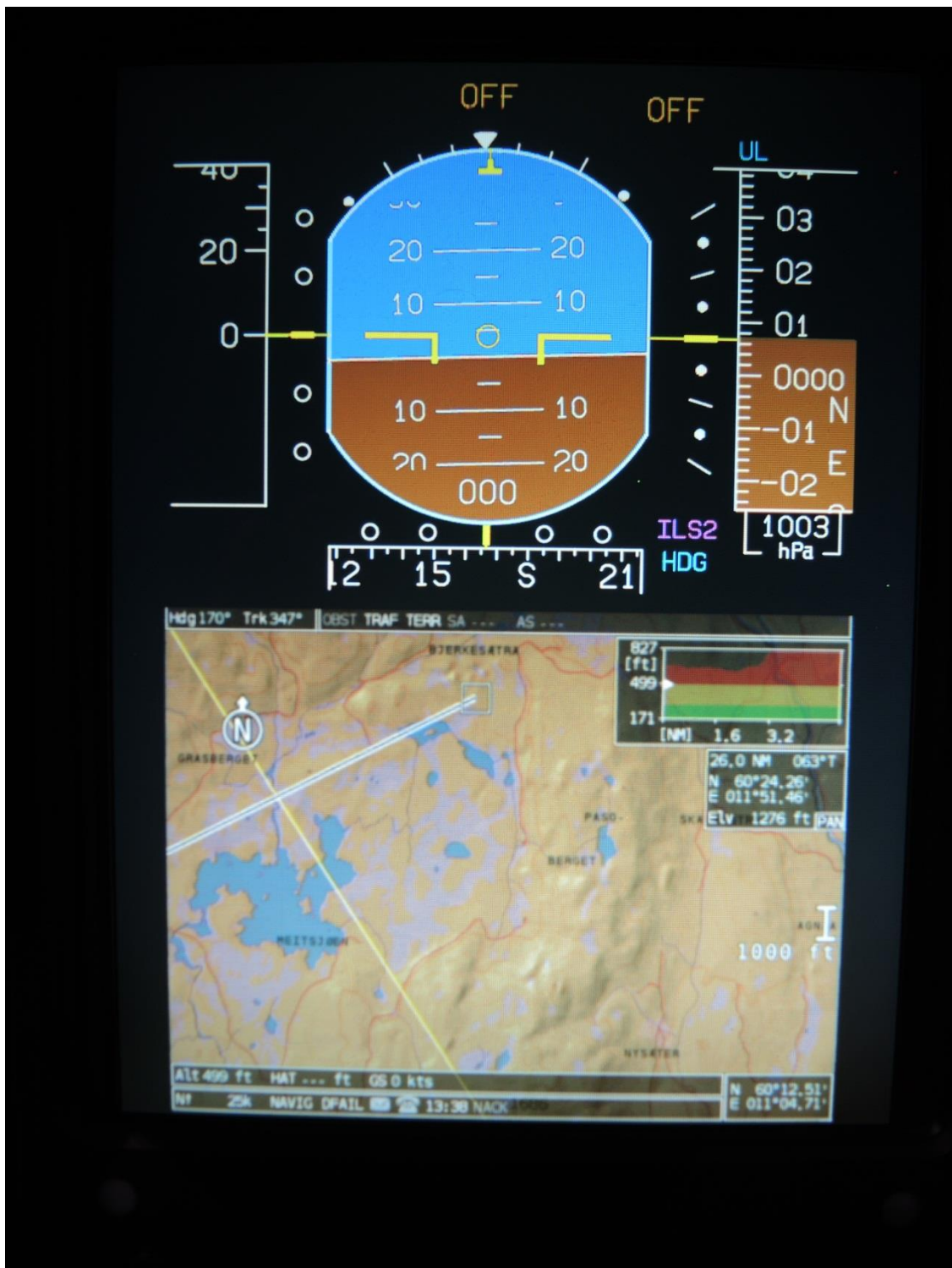
Figure 8: Example of combined display on the HEMS crew member's display with flight instruments on the top and the moving map on the bottom. Photo: AIBN
