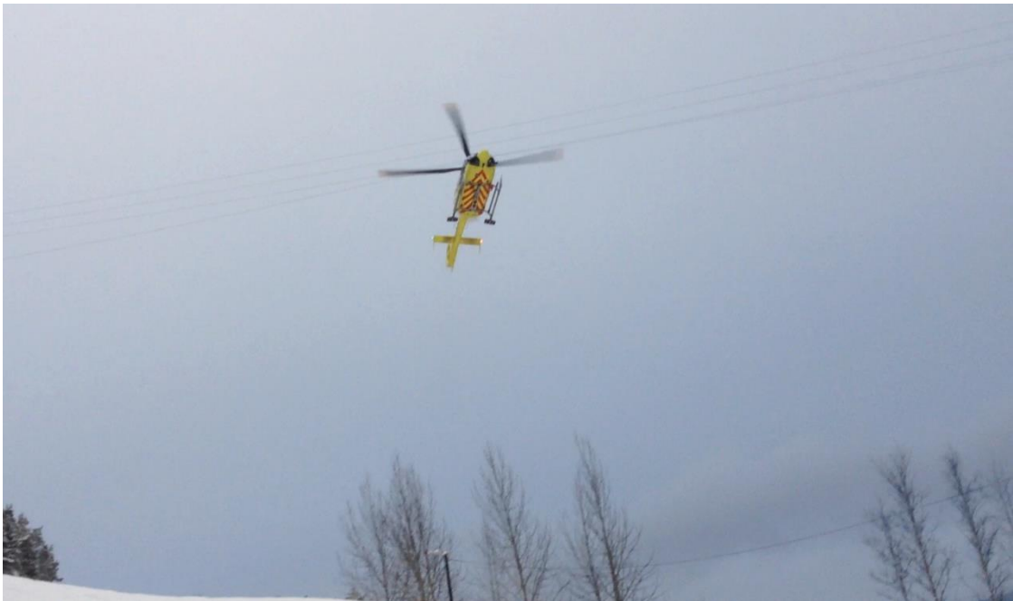
Figure 2: The helicopter has hit the lower line with the wire cutter and pulled it in the direction of flight. The main rotor rotate under the live lines. The line between the street lights along the E16 entry ramp is visible in the bottom of the photo. Photo: Still image from a private video recording
