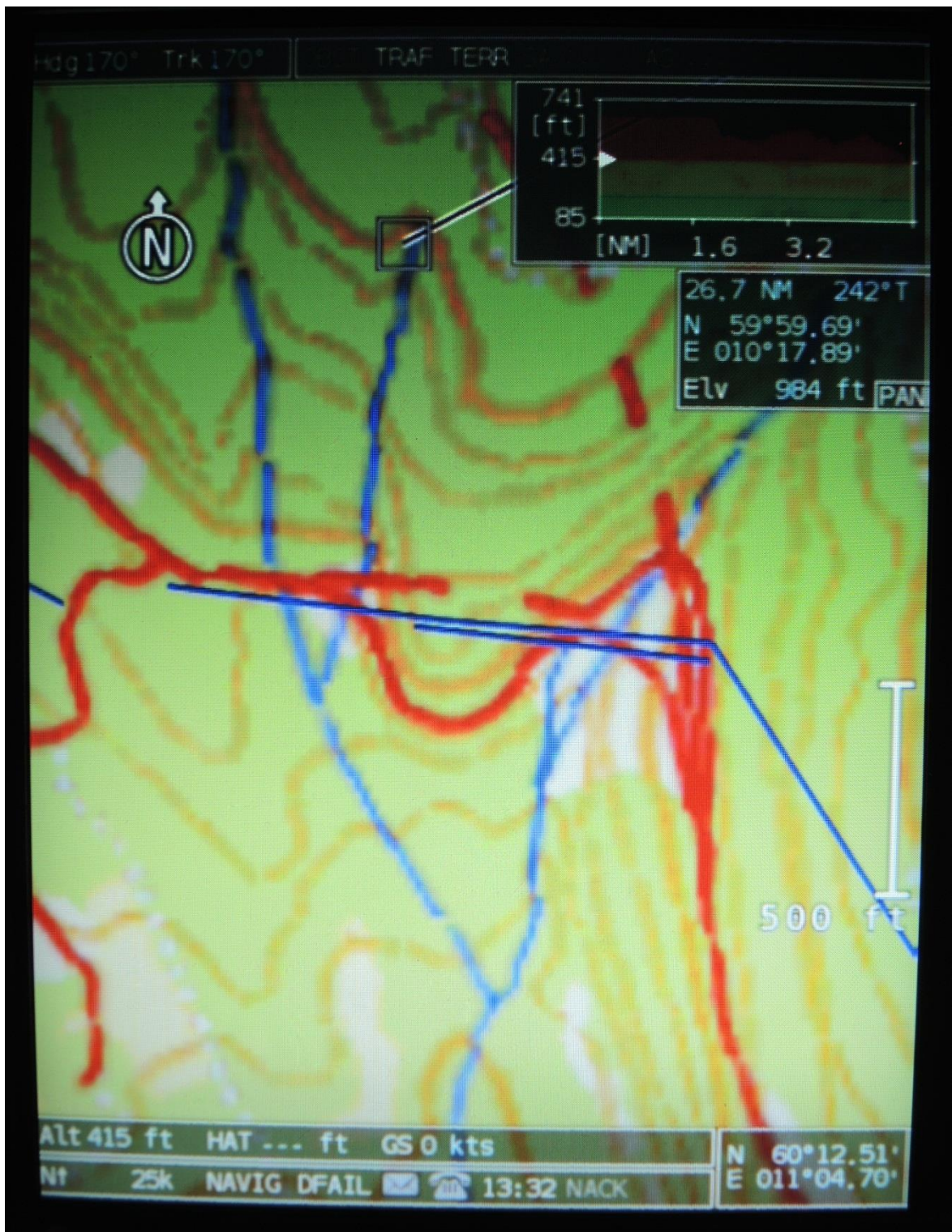
Figure 10: Segment from the same map as Figure 9 with maximum zoom. The presentation seemingly indicates two overhead lines. There is really only one power line, but with data collected from two different databases that both contain inaccuracies. Photo: AIBN
