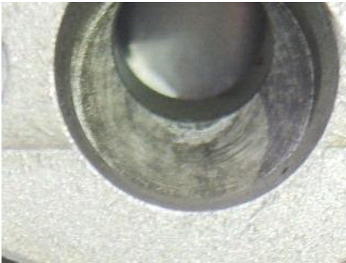
Figure 21: Mark in fuel inlet heat exchanger. Photo: AIBN
