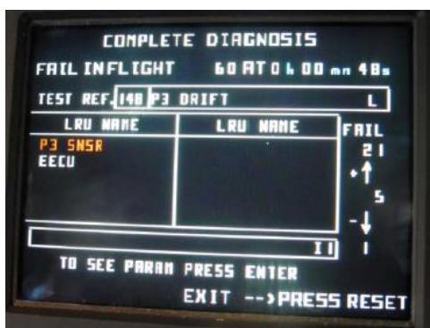
Figure 11: P3 sensor failure VEMD. Photo: Airbus Helicopters
