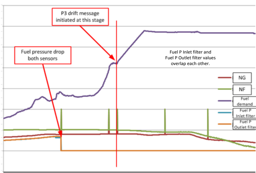
Figure 12: Graph with FADEC parameters. The five peaks on the NF and NG parameters are probably signal failures, and can be disregarded. Source: Turbomeca
