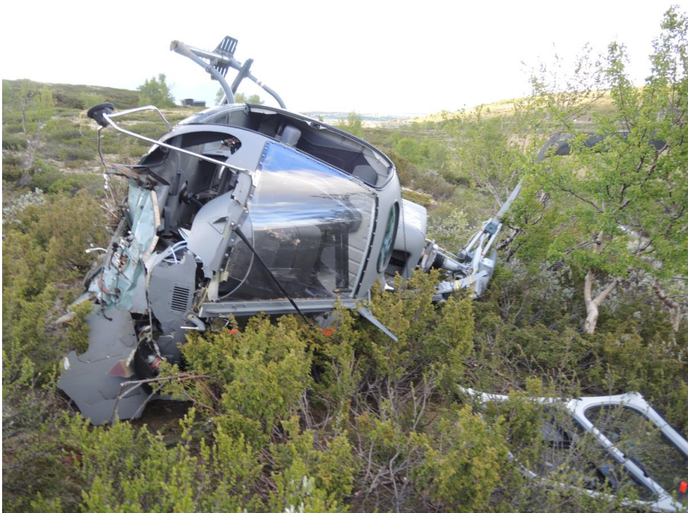
Figure 16: Damages in the nose section. Photo: AIBN
