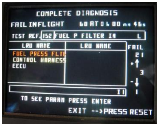
Figure 9: Fuel Press. failure report VEMD. Photo: Airbus Helicopters
