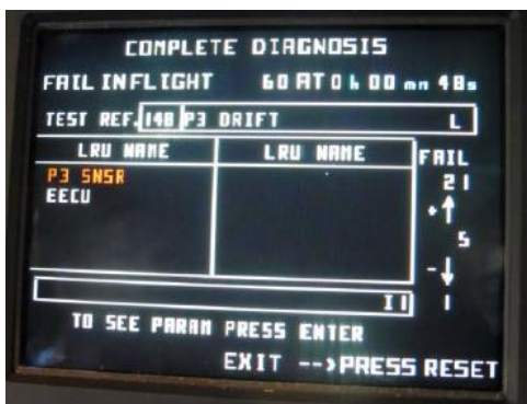
Figur 11: P3 sensor feil VEMD. Foto: Airbus Helicopters
