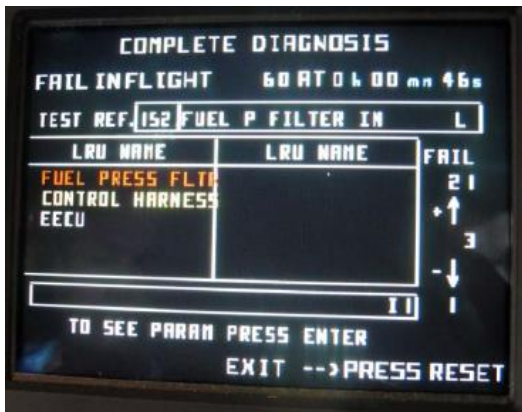
Figur 9: Fuel Press. feilrapport VEMD. Foto: Airbus Helicopters
