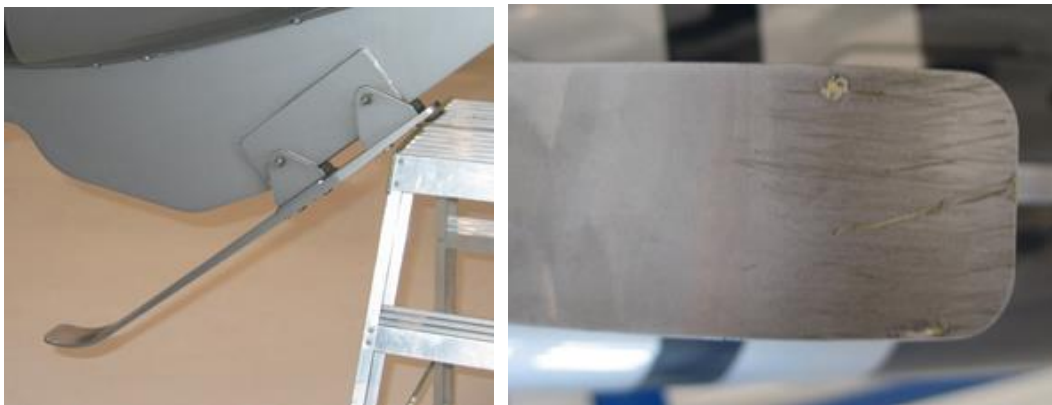
Figure 14: Skid underneath tail structure. Photo: BEA
