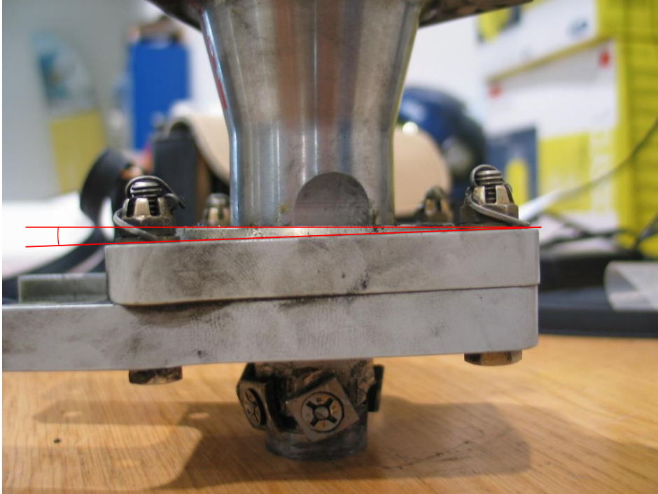
Figure 7: Bearing no. 1, clamped between Bearing Drive and Bearing Flange. Angular discrepancy marked with red lines. Photo: AIBN
