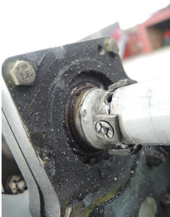
Figure 4: Fracture in the rivet joint on the intermediate tail rotor shaft section installed in LN-ORR. Photo: AIBN
