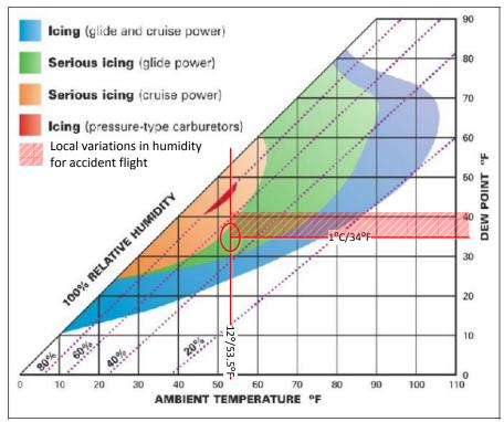
Figure 3: Diagram for air humidity and risk of carburetor ice. The prevailing local conditions at the time of the accident have been entered as red markings and a shaded field. Source: FAA
