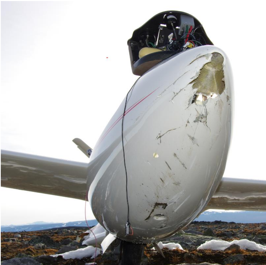
Figure 12: Damage on the sailplane's nose section. Photo: Gudbrandsdal police district
