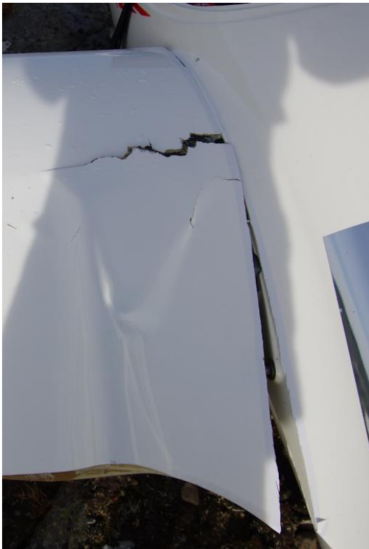
Figure 11: Damage to left wing root. Photo: Gudbrandsdal police district
