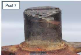
Mechanical damage consistent with gear teeth impressions on three posts
