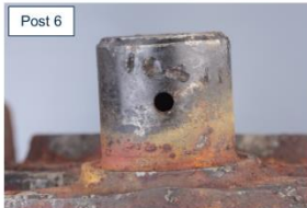
Symmetrical deformation of carrier around post of fractured gear
