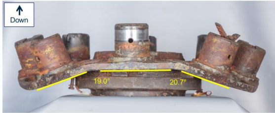
Symmetrical deformation of carrier around post of fractured gear
