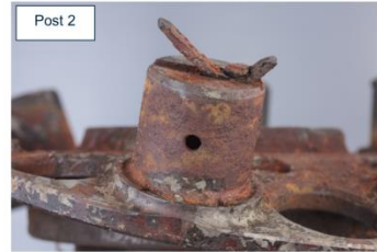
Only one of the planet gear locking tabs remaining attached
