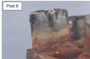
Mechanical damage consistent with gear teeth impressions on three posts
