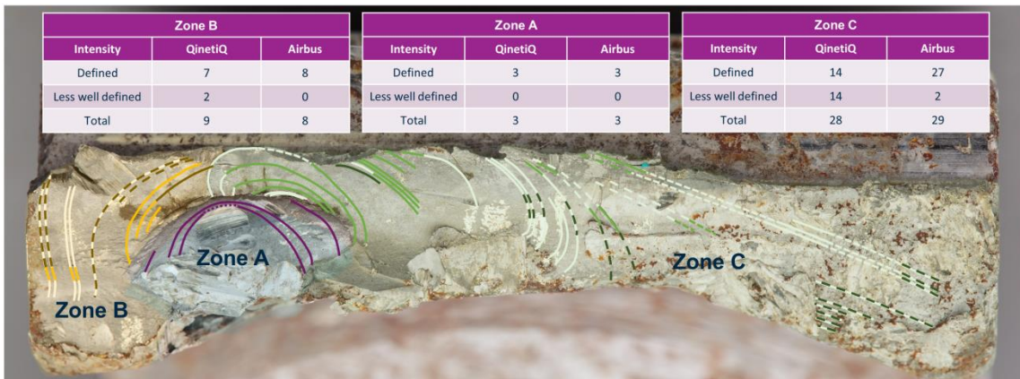
Summary of macro mark observations, solid line – well defined, dashed line – less well defined, see reference [1] for further details. A number of attempts were made to correlate the macro marks with flight data, including engine stop starts, take-off and landings etc. No successful correlations were made.
