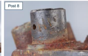
Only one of the planet gear locking tabs remaining attached
