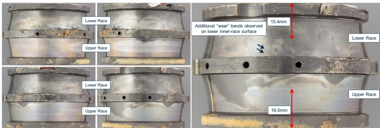
Circumferential "wear" bands observed on the inner-race surfaces
