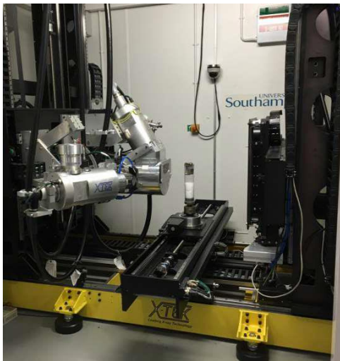
Figure 37: The x-ray tomography set up. The part to be scanned is in the tube in the centre of the figure. Photo: AIBN
