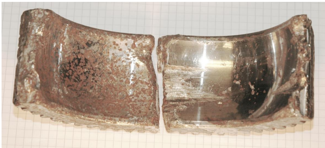
Figure 27: The two fractured gear segments. Appearance of wear marks on the right, while not on the left indicate separation while other parts still have been in motion. Photo: AIBN/NDL
