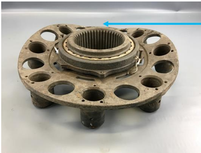
Figure 49: The second stage planet carrier found in February 2017 shown after cleaning. The lower mast bearing is shown on top of the carrier. Photo: AIBN/QinetiQ
