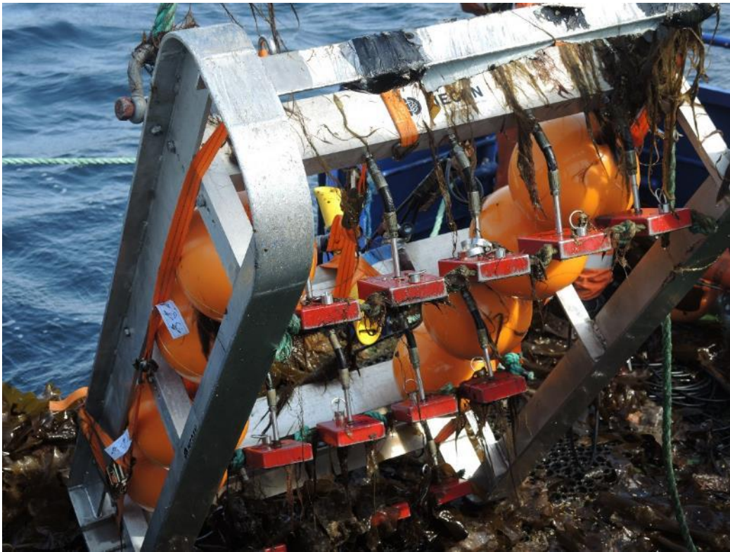
Figure 63: The magnetic sledge being retracted from the sea. Photo: AIBN
