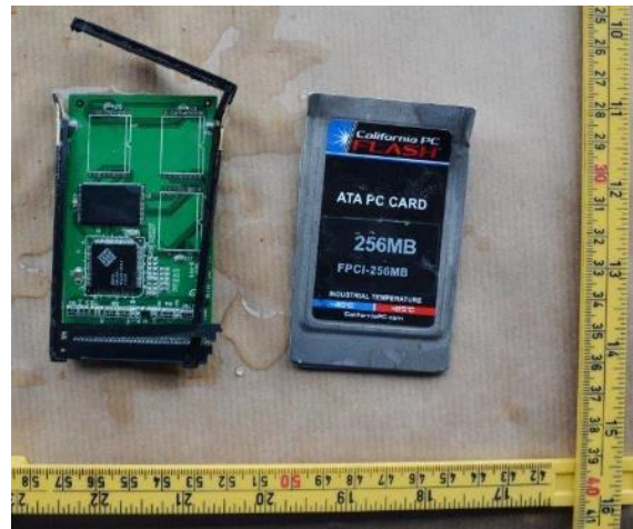
Figure 15: M^ARMS PCMCIA card. Photo: AIBN
