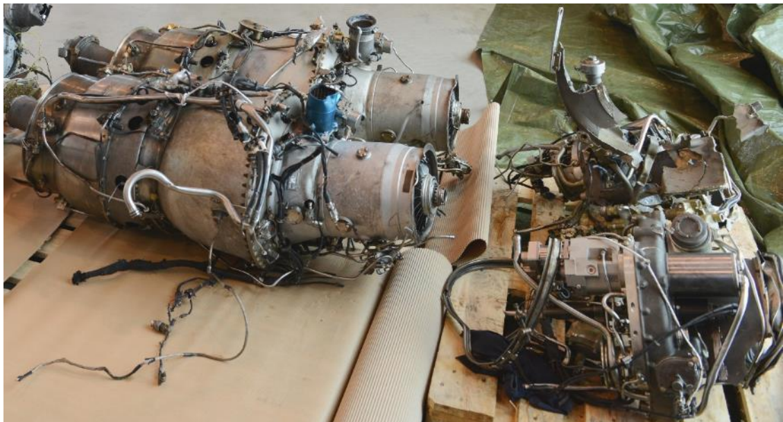
Figure 23: The engines at the AIBN hangar. They had similar damages to a large extent. Both intake sections (Module M01) which had separated from the front part of the engines can be seen to the right of the photo. Photo: AIBN
