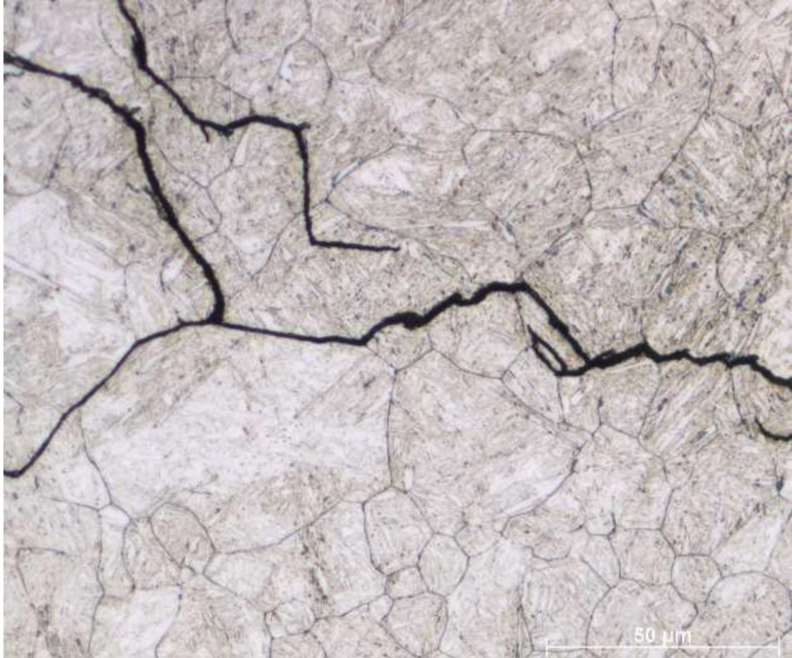
Figure 41: The sub-surface crack propagation is both trans- and inter-granular. Polished surface etched with saturated Picric acid solution (with HCl). Roller direction to the left. Photo: AIBN/QinetiQ
