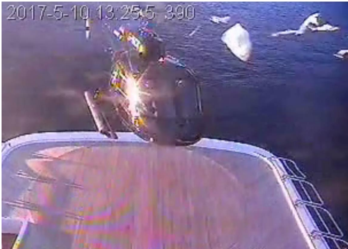
Figure 1: The helicopter as the tarpaulin hit the main rotor. Photo: CCTV M/Y Bacarella
