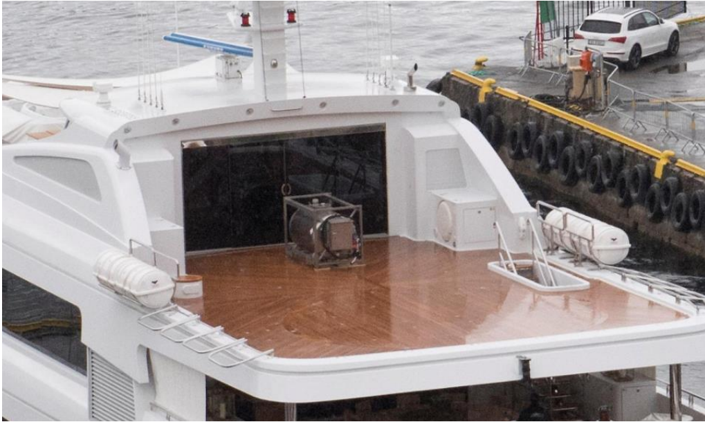
Figure 4: Helideck on M/Y Bacarella with provisional jet fuel bowser. Photo: Bergensavisen newspaper
