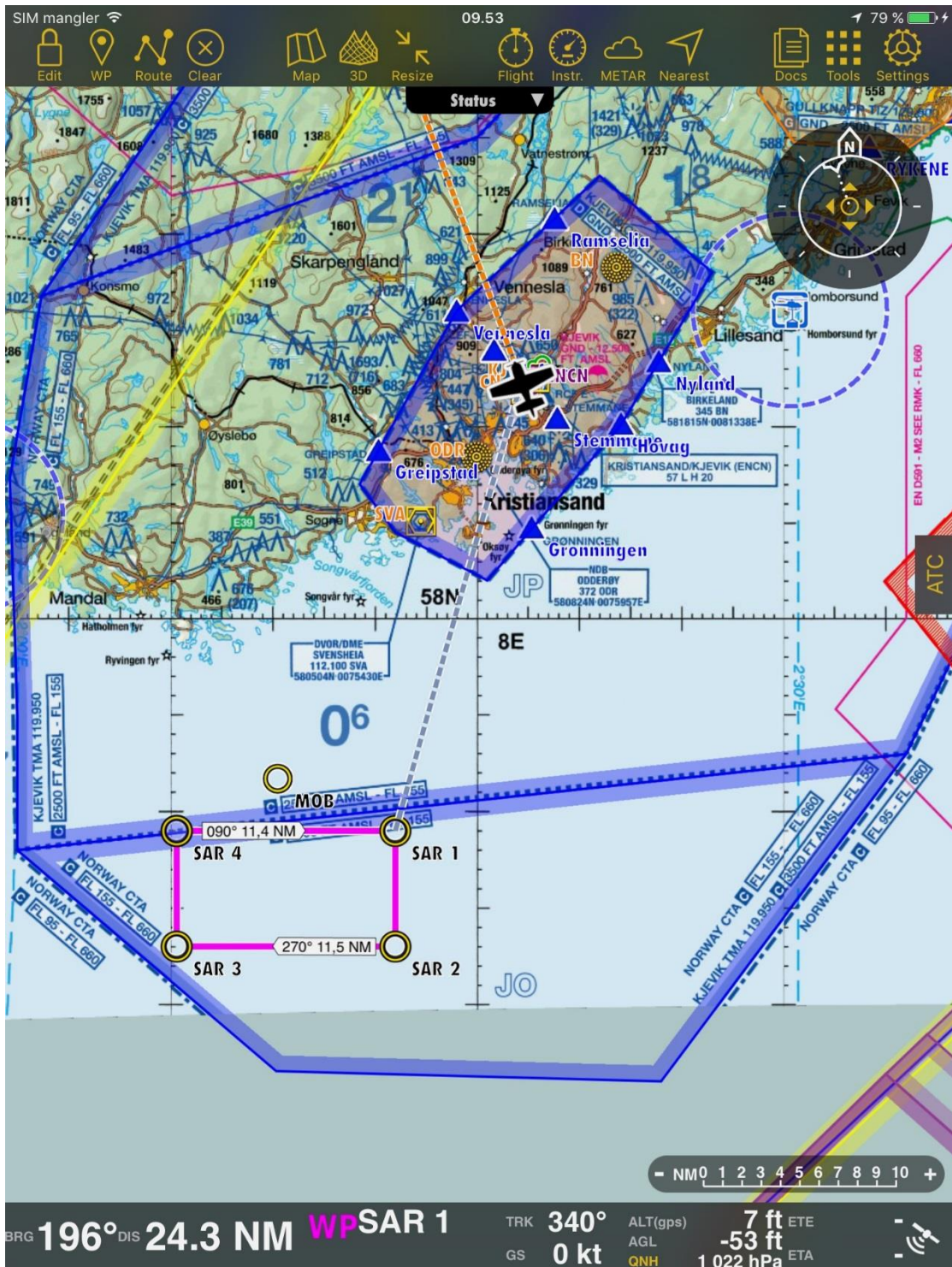
Figure 1: Tablet screen shot showing the Air Navigation Pro software with the search area coordinates (magenta) and the course from Kjevik Airport. The Kristiansand Airport Kjevik (ENCN) control zone is indicated in blue (the smallest area around the airport). Source: Air Navigation Pro screen shot
