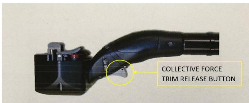
Figur 14: Collective med collective force trim release button. Foto: S-92 Pilot training manual/SHK
