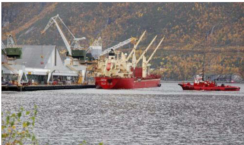
Figure 12: A tugboat assists in keeping the ship clear of the quay since the draught is too great. For ships with an equivalent load capacity to the Federal Kivalina, 6000-9000 tonnes of aluminium oxide are usually unloaded, and it may take up to 24 hours before the ship can lay alongside the quay. Photo: Aura Avis
