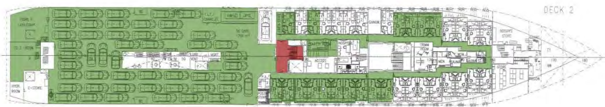
Figure 31: Registered soot deposits on deck 2 (green: no spread of smoke; red: moderate to heavy spread of smoke; white: uninspected area).
