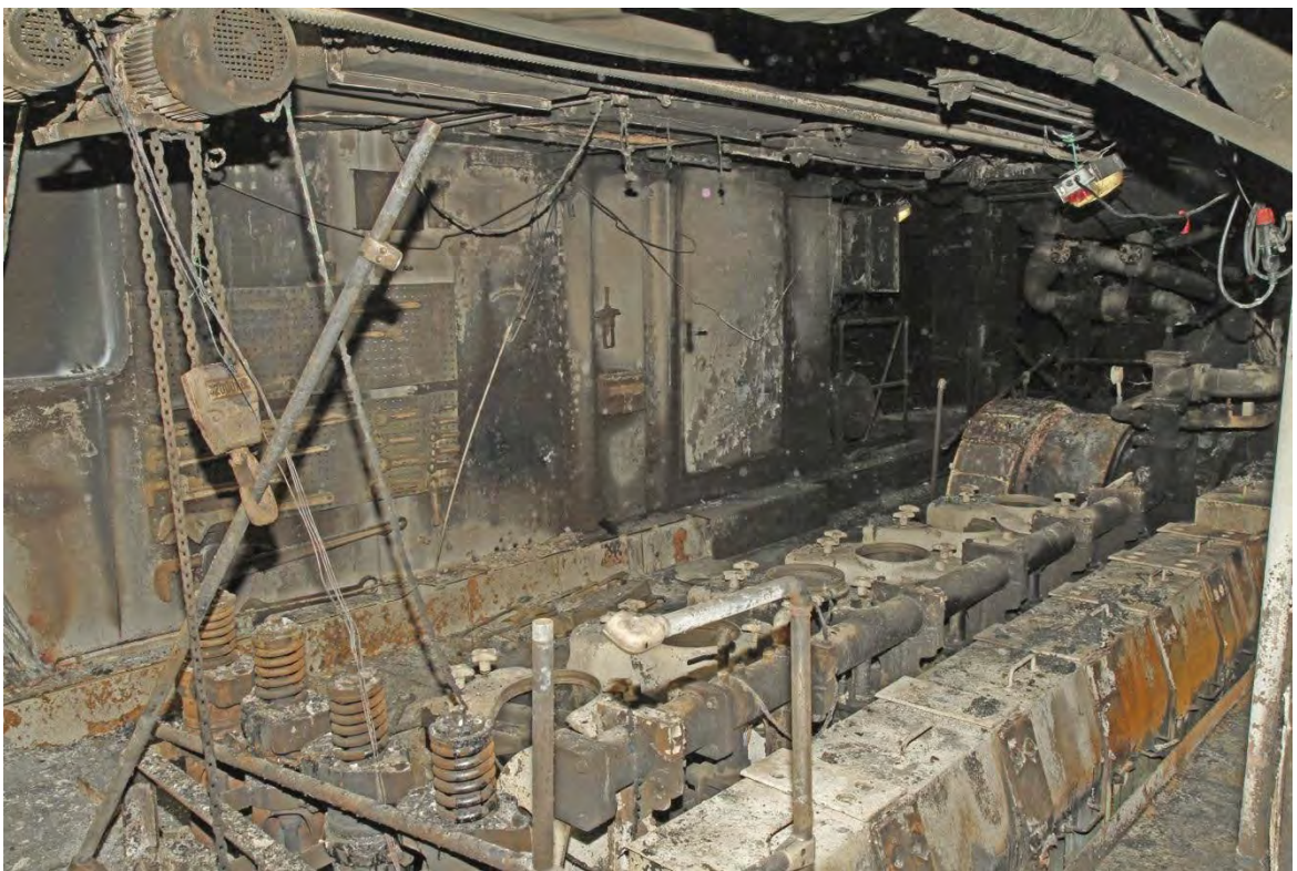
Figure 4: Starboard side of the main engine room looking aft from the forward gallery. The top of the starboard main engine can be seen in the foreground. The bulkhead dividing the workshop from the engine room can be seen in the background, with the aft entrance door in the middle of the photo. Photo: The police.
