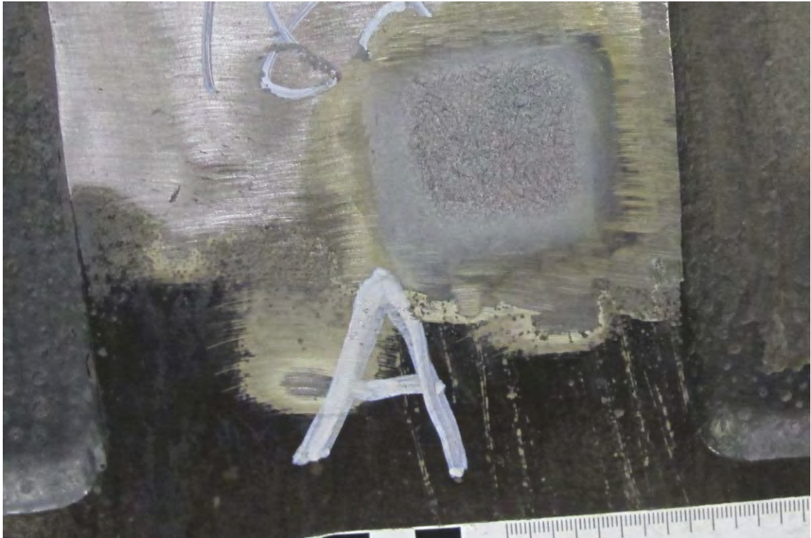
Fig. 5 Close-up of area A prepared and etched for examination in the portable microscope and finally hardness measurements. The area is representative for the areas Ref., B, C and D.
