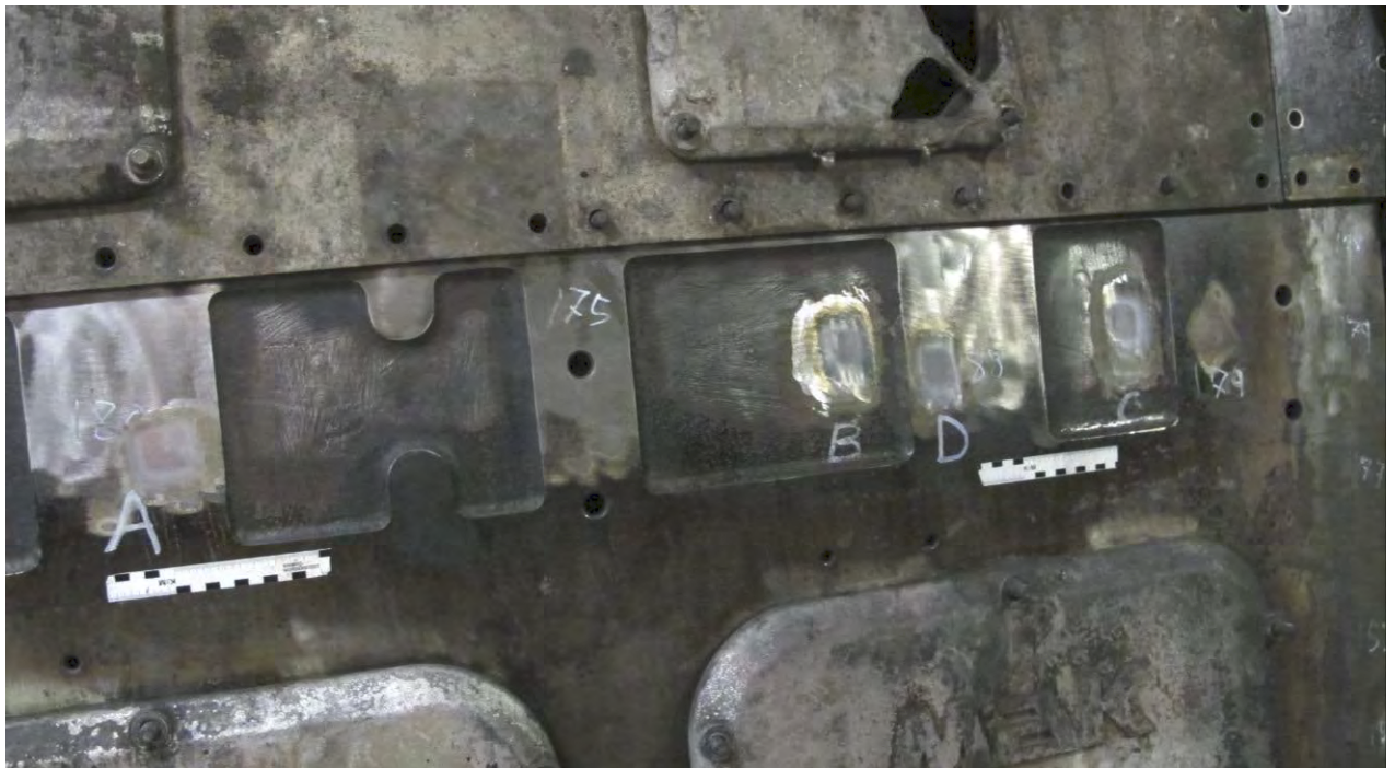
Fig. 4 Overview of the prepared areas for examination the microstructure and hardness measurements.
