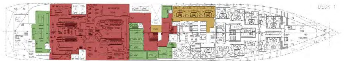
Figure 30: Registered soot deposits on deck 1 (green: no spread of smoke; orange: some spread of smoke; red: spread of moderate to heavy smoke; white: uninspected area).
