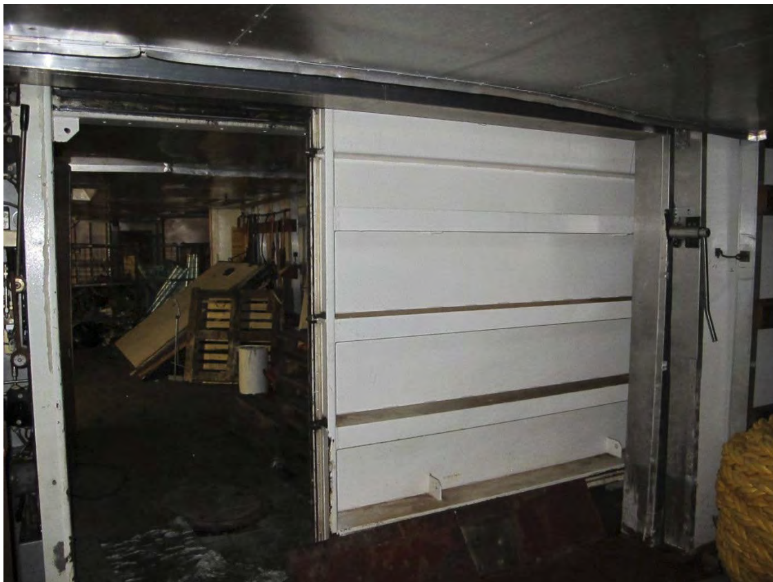
Figure 39: The photo shows the watertight sliding door between cargo hold no 1 and cargo hold no 2. The investigation found wear on seals on the underside of the door. Photo: AIBN.
