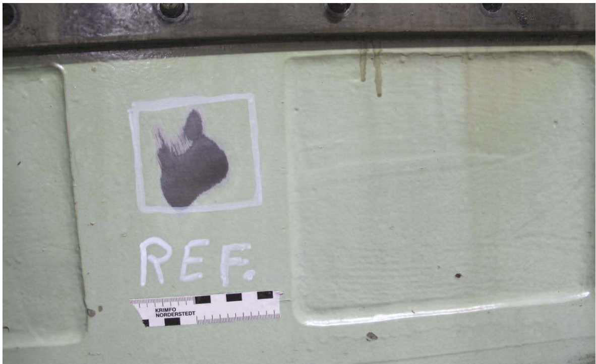
Fig. 6 Close-up of the reference area (ref. to Fig. 1) used for comparison of the microstructure and hardness values.
