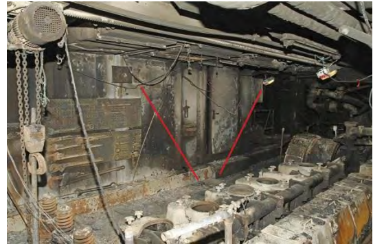
Figure 43: The top of the starboard engine looking aft at an angle. The bulkhead with the aft door to the workshop can be seen in the background. The fire has left an upward V-shaped mark. Photo: The police.
