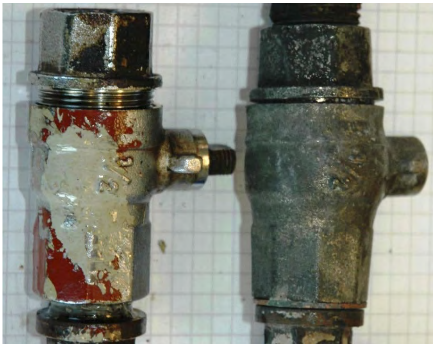
Figure 22: Ball valve from drainage pipe. The reference valve on the left was installed on Nordlys' port main engine, while the valve on the right was installed on Nordlys' starboard main engine. Photo: The Norwegian Armed Forces' laboratory service.
