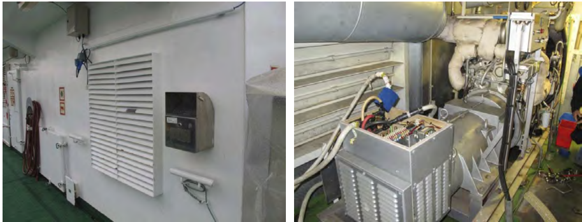
Figure 26: The photo on the left shows the aft damper in the generator room, viewed from the outside. The photo on the right shows the starboard damper viewed from inside the emergency generator room. Photo: AIBN.
