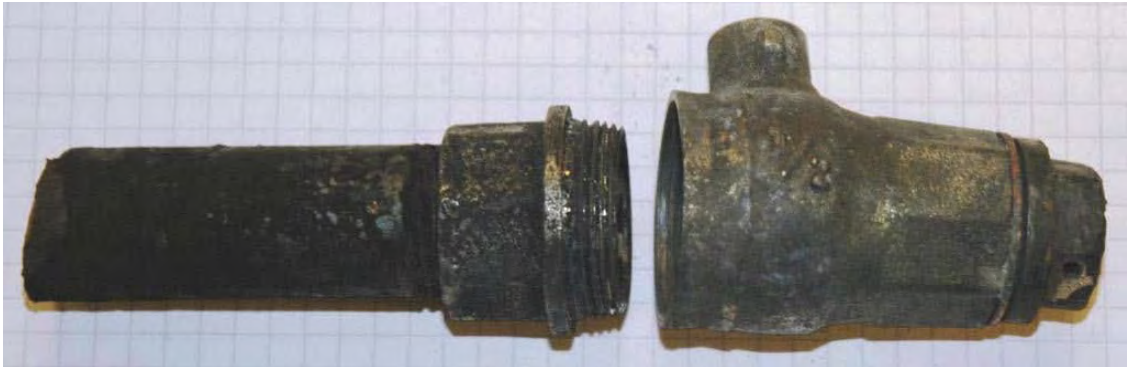
Figure 21: Drainage valve disconnected from the starboard engines. Photo: The Norwegian Armed Forces' laboratory service.
