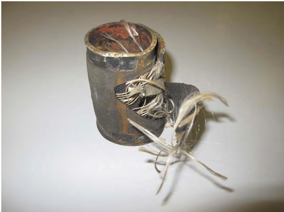
Figure 25: The photo shows the ruptured cooling water hose. Photo: AIBN.
