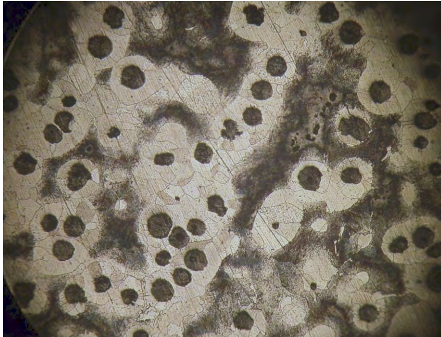
Fig. 9 Area B, representative also for area C. The prepared area shows a microstructure characteristic for nodular cast iron as expected. The microstructure consists of ferrite and pearlite with spheroidal graphite. Compare to the reference area it is observed somewhat more ferrite. Modification of the microstructure due to heat affection was not observed. Magnification 100 X.
