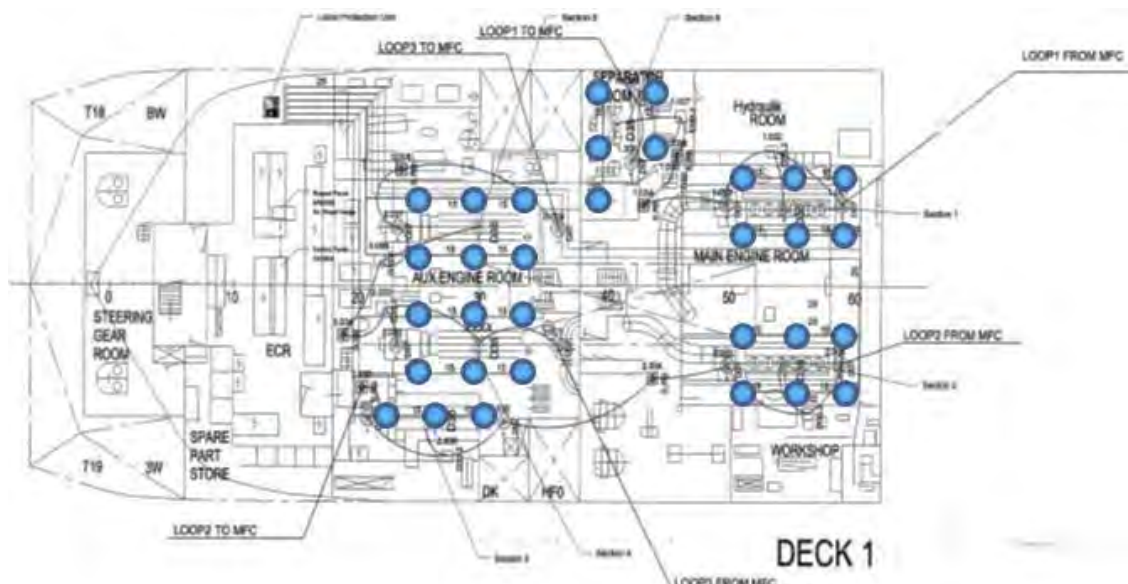
Figure 12: Sketch showing the position of the nozzles in the local application fire-extinguishing system. The nozzles (marked as blue bullet points) are placed above each main engine (six per engine), in the separator room (five), above each auxiliary engine (six per engine) and above the boiler (three). This adds up to a total of 32 nozzles on deck 1 (under deck 2). There are no nozzles at the tank-top level.
