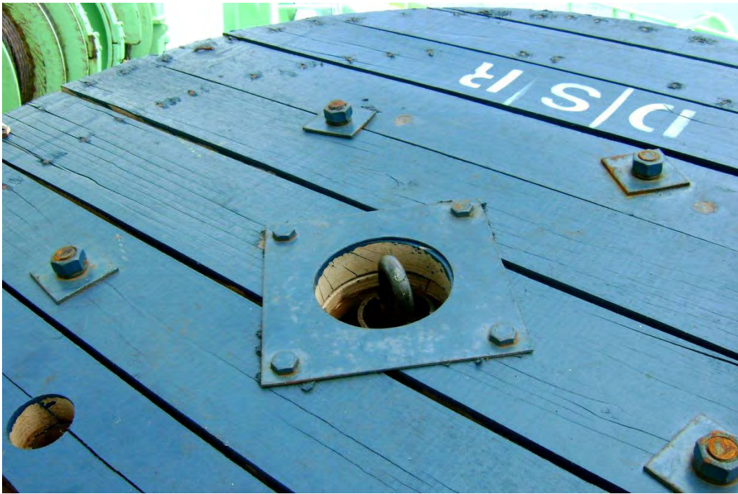
Figure 6: Steel-cross stand viewed from the top of a drum. Photo: BW Suez Everett
