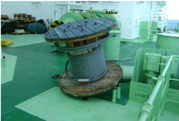
Figure 4: Drum with 15 turns of wire left, stopped against the port bollard in the Grand Canyon. Photo: BW Suez Everett
