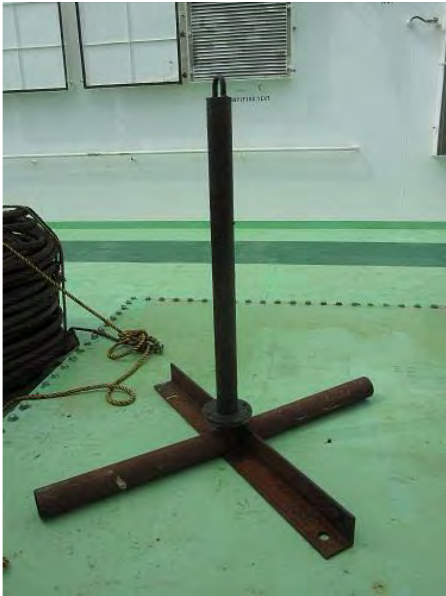
Figure 5: Steel-cross stand for wire drums. Photo: BW Gas.
