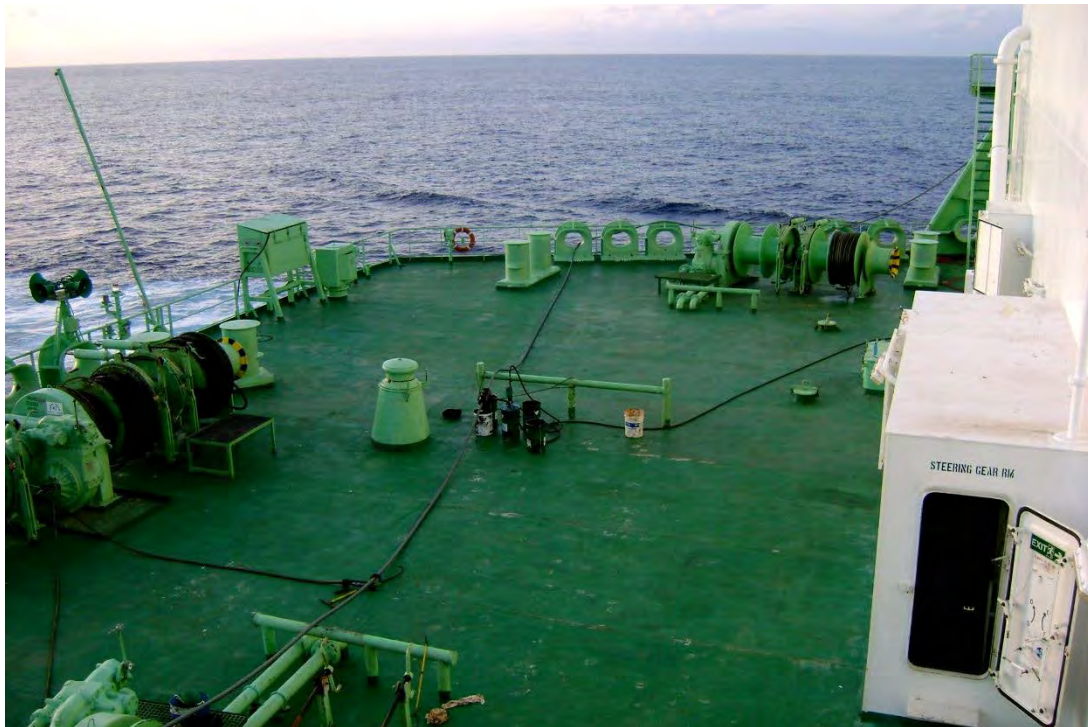
Figure 8: View of the port side of the poop deck, with wire pulled through the port mooring hole aft and across the deck to the starboard mooring winch. Photo: BW Gas.
