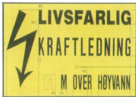
Figure 14: Warning sign where overhead cables span the fairway. Source: Regulations relating to beacons, seamarks etc. Annex A4
