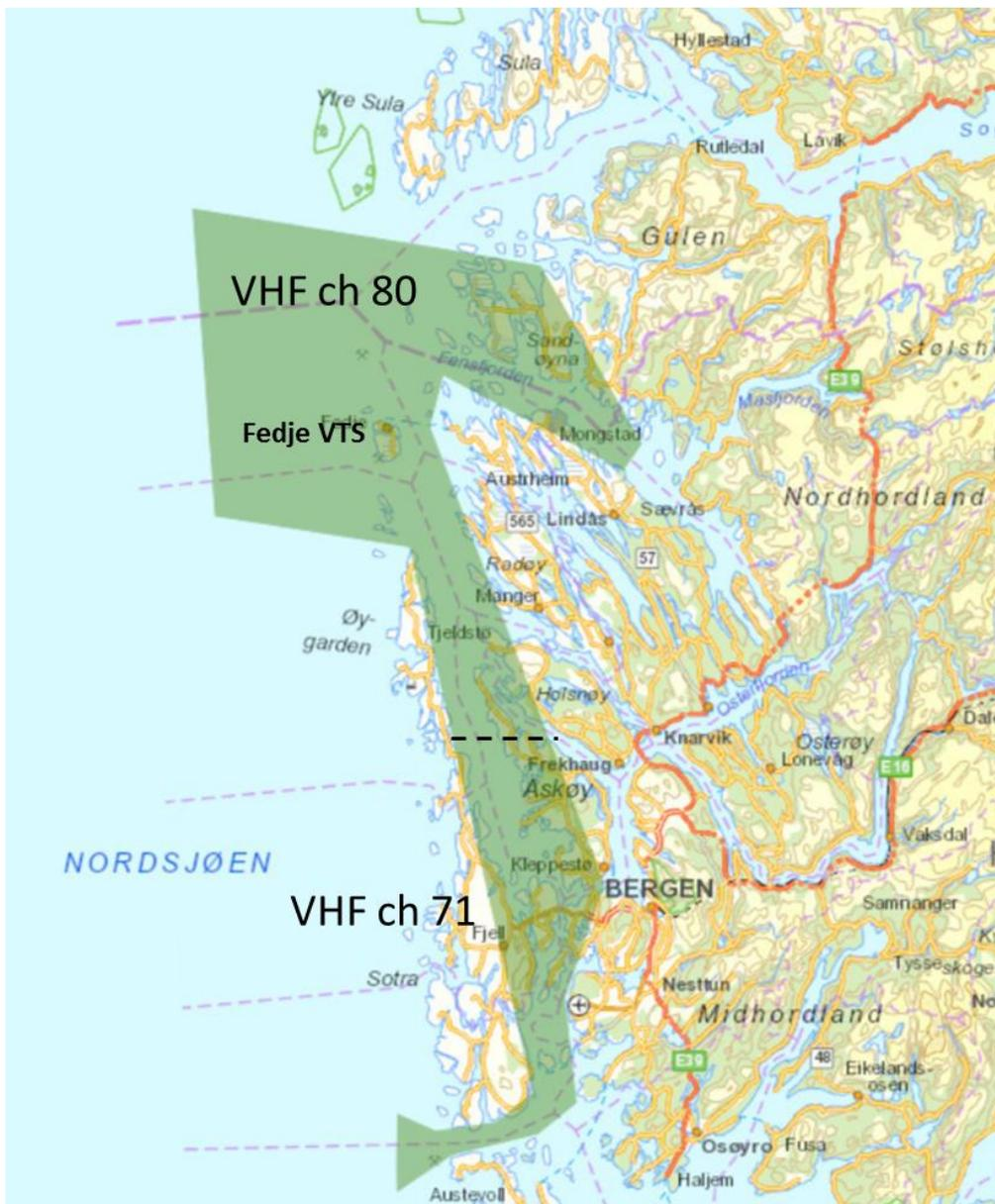
Figure 39: The Fedje VTS area and overview of working channels to be used for VHF radio communication. Map: The NCA
