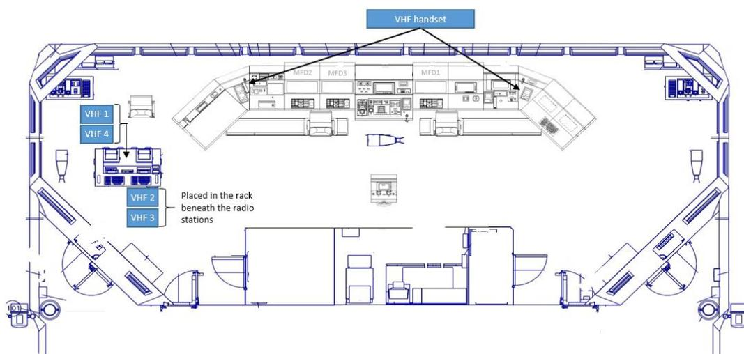
Figure 26: Bridge design on HNoMS Helge Ingstad. Position of VHF radios. See Figure 3 for information about the bridge team’s positions on the night of the accident. Illustration: The Royal Norwegian Navy/AIBN
