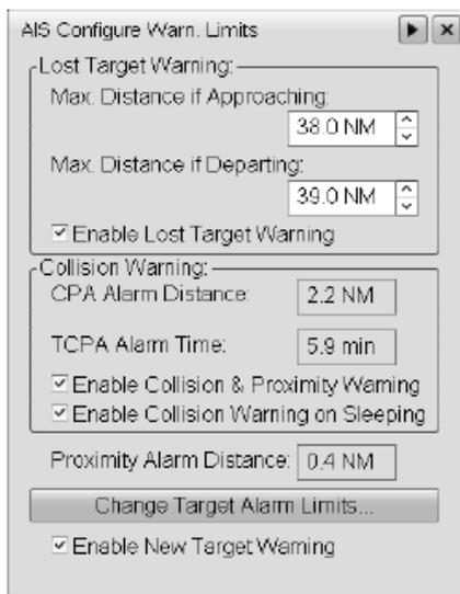
Figure 31: The function for warnings about sleeping AIS targets is activated by ticking the box 'Enable Collision Warning on Sleeping'. The settings for receiving warnings can also be changed. Source: The Norwegian Navy
