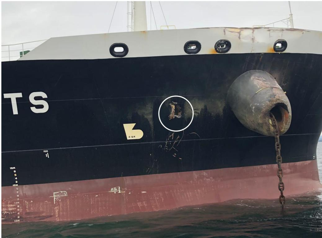
Figure 21: The hawsepipe and the damage sustained by Sola TS in the collision. The hole in the hull is marked with a white circle. Photo: The Norwegian Maritime Authority
