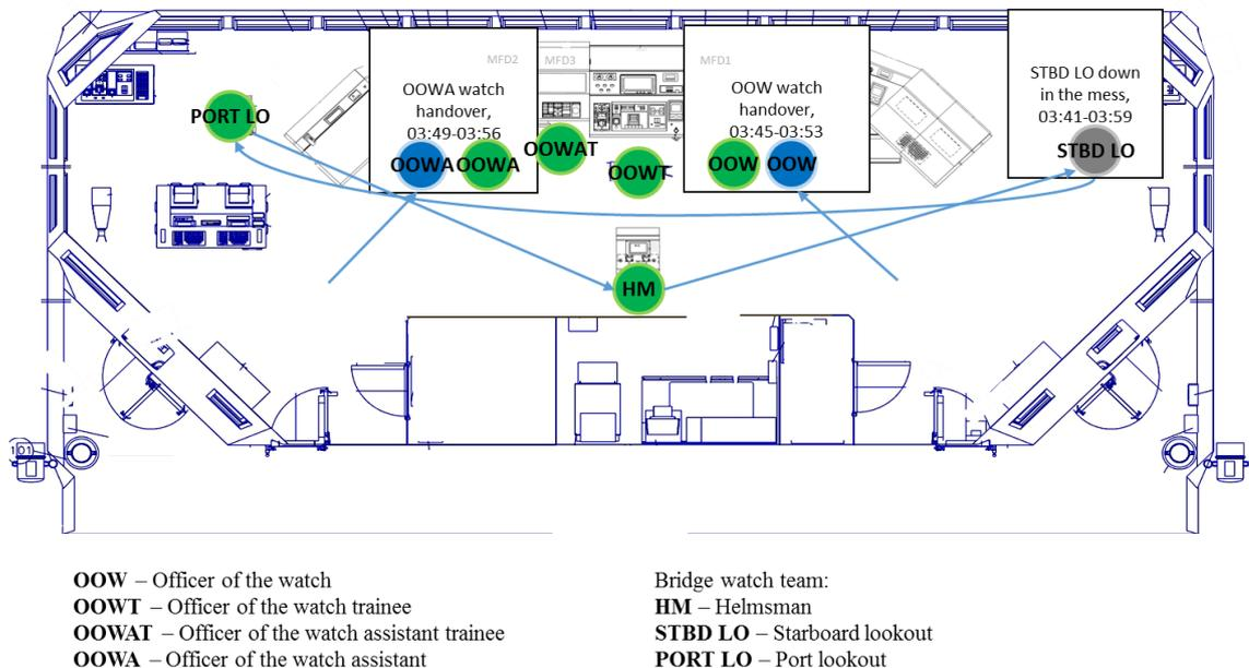
Figure 9: Crew on the bridge of HNoMS Helge Ingstad during the period from 03:40 to 03:59, a period of watch handovers and bridge watch team rotation, when the starboard lookout had gone down to the mess. Illustration: The Royal Norwegian Navy/AIBN
