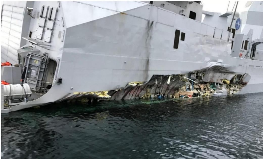
Figure 20: Damage to the hull along the starboard side of HNoMS Helge Ingstad after the collision. Photo: The Norwegian Coastal Administration
