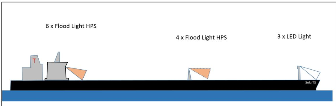
Figure 36: Simplified drawing of the forward-pointing deck lights that were lit on departure. Shortly after departure, the four midship lights were turned off. Illustration: Tsakos Columbia Shipmanagement S.A./AIBN
