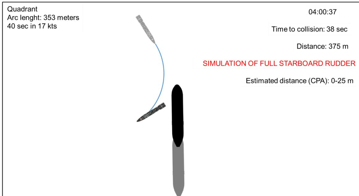
Figure 43: Had HNoMS Helge Ingstad made a manoeuvre to starboard 38 seconds before the collision, the collision would probably have been avoided. The vessels would then have passed each other port to port with a CPA of approximately 0 - 25 m. Illustration: Safetec/AIBN
