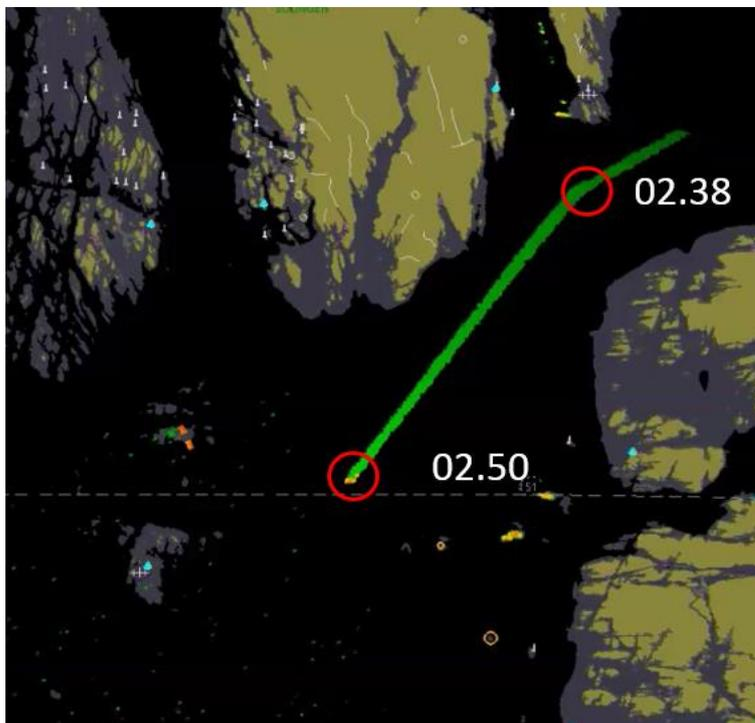
Figure 4: Screenshot of radar replay from Fedje VTS showing the position of HNoMS Helge Ingstad at 02:38 and 02:50, respectively. The broken line represents the boundary of the Fedje VTS area. Note: When preparing the radar replay after the accident, an artificially long afterglow was used to illustrate the frigate's voyage. Source: The NCA/AIBN
