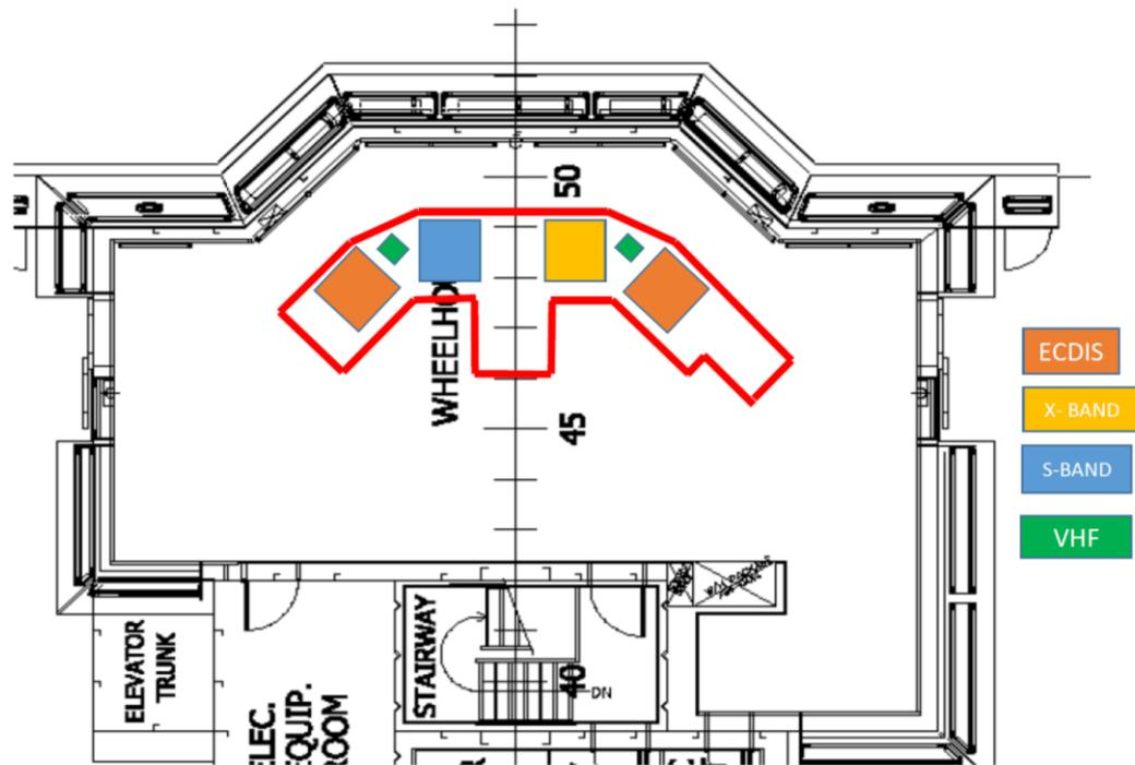
Figure 34: Bridge design of Sola TS. Illustration: Tsakos Columbia Shipmanagement S.A.
