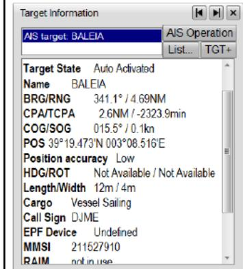
Figure 30: By placing the marker on the target and pressing 'DATA', a pop-up window will appear with information about the target's name, bearings, distance, course, speed etc.
