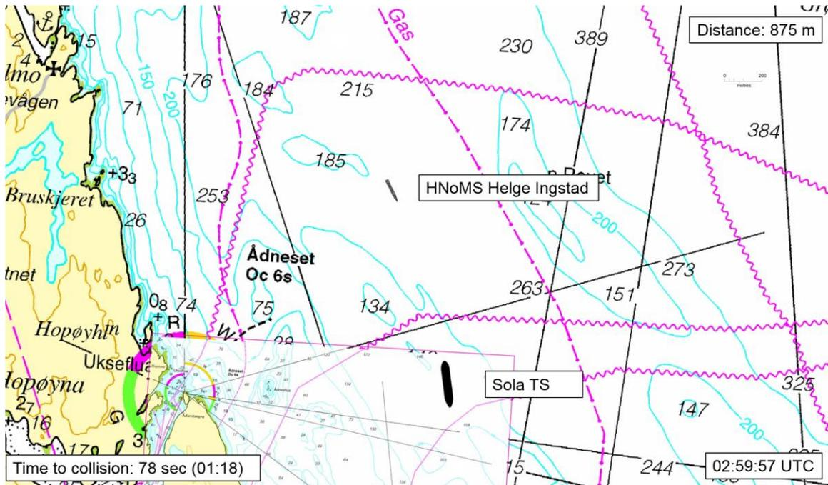
Figure 16: At 03:59:57, there was a distance<sup>14</sup> of approximately 875 metres between 'HNoMS Helge Ingstad' and Sola TS. Illustration: Safetec/AIBN
