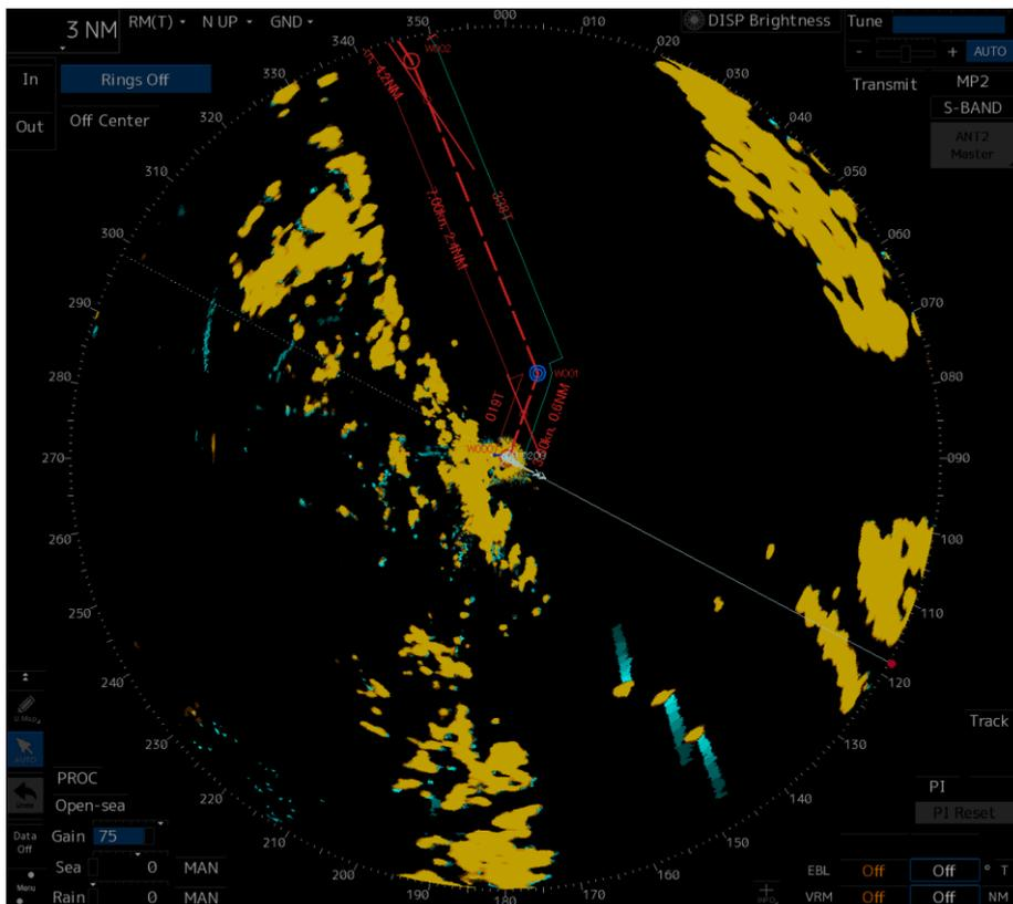
Figure 10: At 03:45, the S-band radar on Sola TS, set to a range scale of 3 nm, showed three vessels to the south and none to the north. Source: Tsakos Columbia Shipmanagement S.A.
