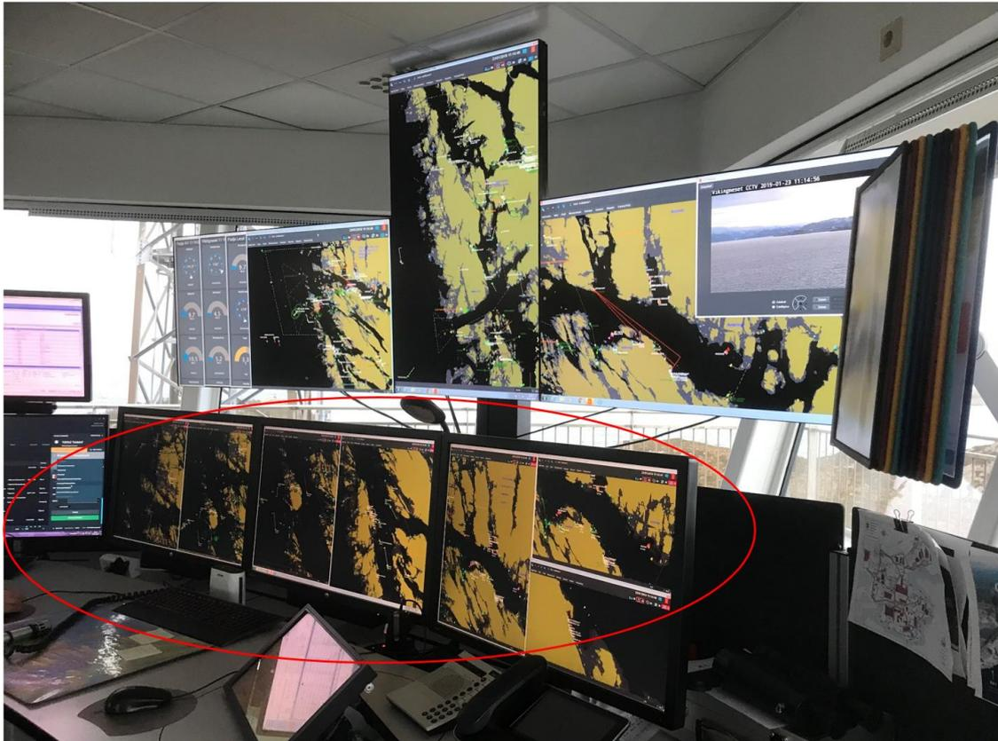
Figure 40: Workstation for the VTS operator monitoring the northern part of the Fedje VTS area. The three 'main screens' are marked with a red circle. The overview screen is placed above the main screens. Photo: AIBN
