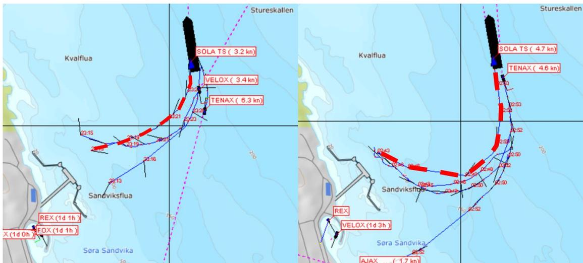
Figure 44: Left: Sola TS manoeuvring out from the quay on the observation voyage. Right: Sola TS manoeuvring out from key the night of the accident. Source: NCA/AIBN
