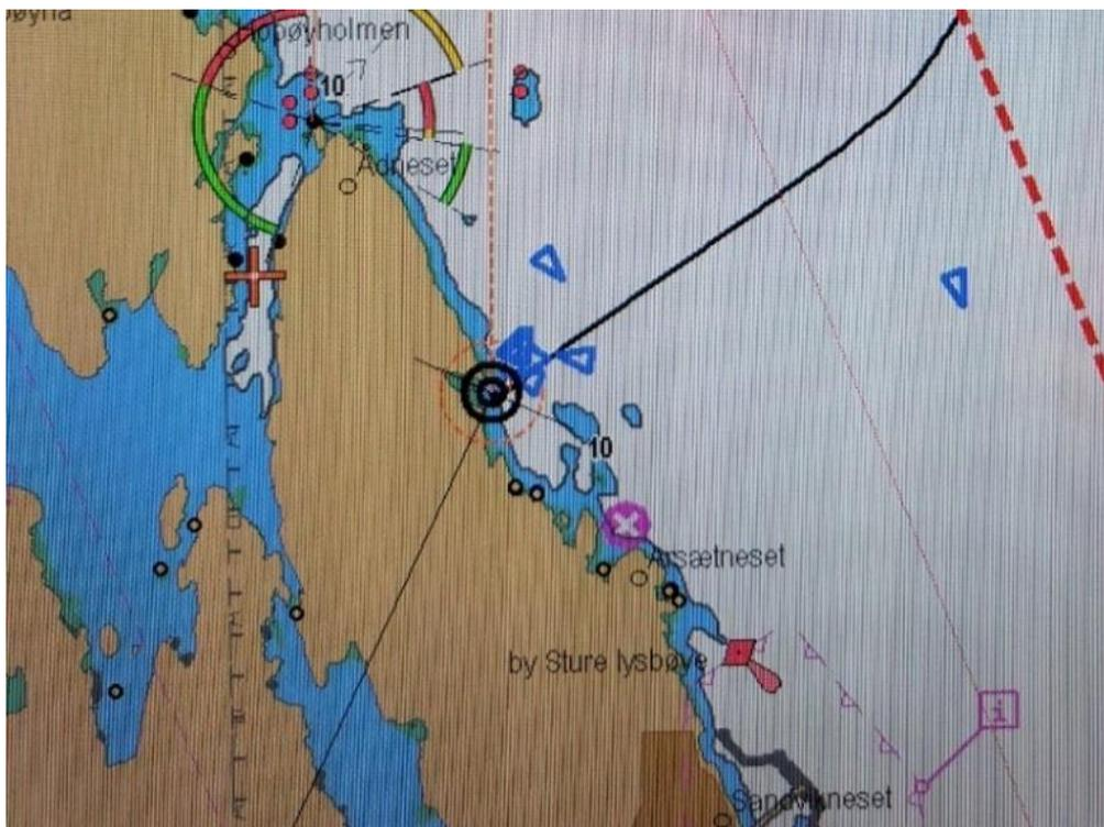
Figure 32: Map section showing the safety zone (marked with a pink broken line in the lower right corner) around the Sture Terminal. Photo of the ECDIS/MFD 3 on HNoMS Helge Ingstad taken after the accident. Photo: Crew member of HNoMS Helge Ingstad
