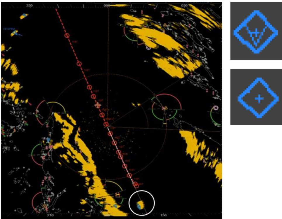
Figure 51: On the left: Screenshot of video recording of radar display on HNoMS Roald Amundsen on the observation voyage. Sola TS with escorting tug marked with a white circle. Virtual navigation object in the top right corner. Navigation object, landmark or buoy with AIS transponder in the lower right corner. Illustration: AIBN
