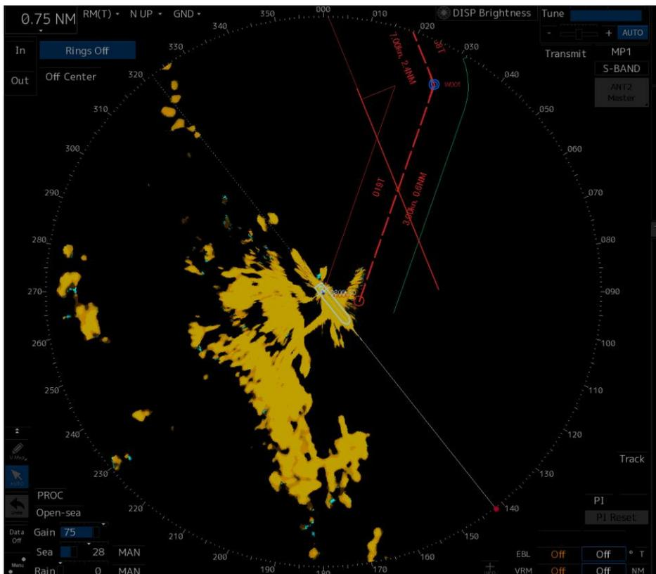
Figure 8: The S-band radar on Sola TS, set to a range scale of 0.75 nm, showed no other maritime traffic at 03:13. Source: Tsakos Columbia Shipmanagement S.A.
