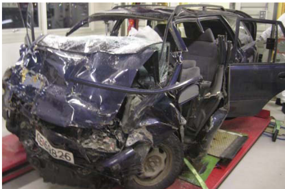
Figure 9: Damage to the front of the Mitsubishi Lancer. Survival space for all seats in the car except the driver's seat.
