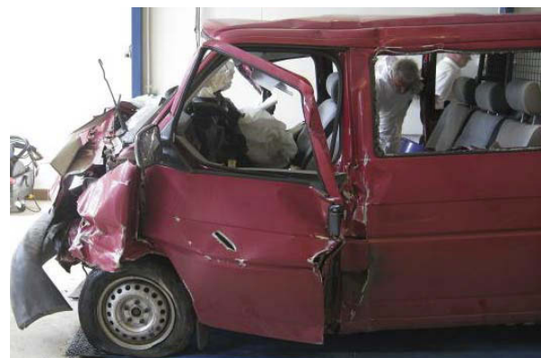
Figure 23: Damage to the front of the VW Caravelle. Survival space for the driver's seat.
