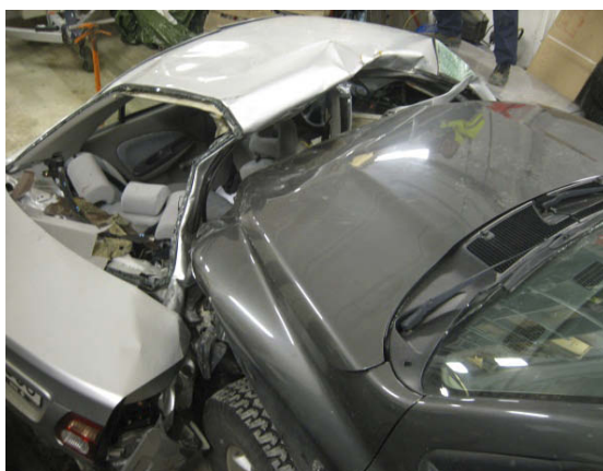
Figure 13: Reconstruction showing the vehicles' positions in relation to each other at the moment of impact.
