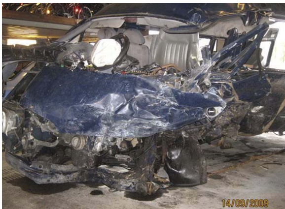
Figure 25: Damage to the front of the Ford Transit (photograph: Norwegian Public Roads Administration). Survival space for all seats in the car, limited space for the driver's seat.
