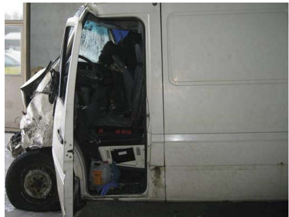
Figure 17: Damage to the front of the Mercedes Sprinter van. Survival space for the driver's seat.
