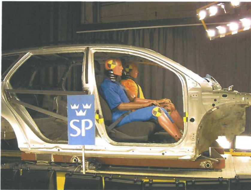
Figure 37: Chassis with dummies before the tests were conducted.
