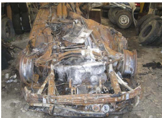
Figure 22: Mercedes E220 completely burned out, no survival space in the car.
