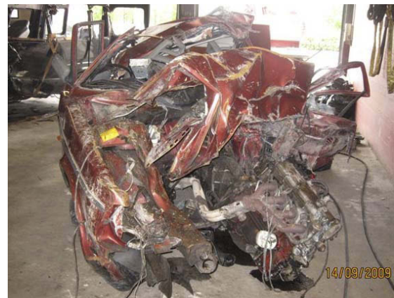
Figure 26: Totally destroyed Volvo 240 (photograph: Norwegian Public Roads Administration). No survival space for the driver's seat.
