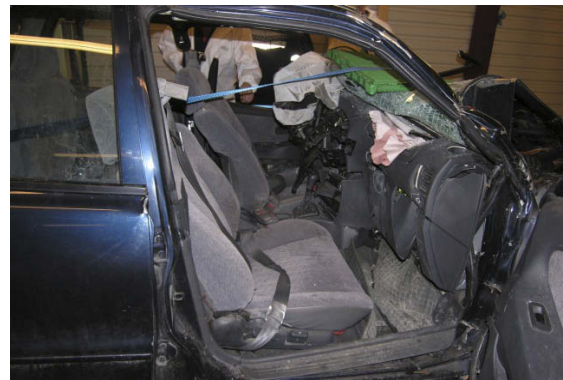
Figure 10: Restricted survival space for the driver's seat.
