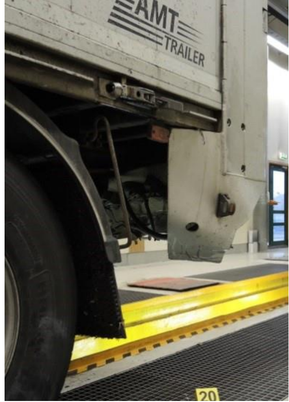
Figure 5: The left side panel is marked by the encounter with the crash barrier on the right-hand side of the opposite lane. Photo: AIBN
