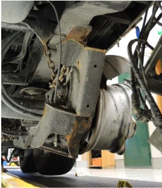
Figure 6: The torn-off left suspension rod on the forward axle. Photo: AIBN
