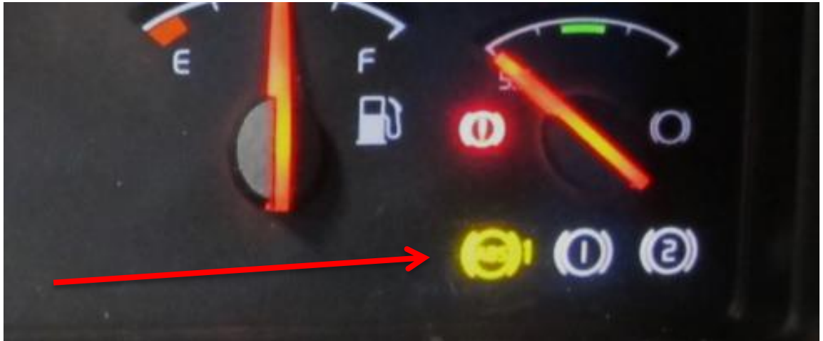
Figure 13: Dashboard display, without ABS power supply fuse for trailer. The yellow warning light means that it is connected to a trailer with ABS fault. (The arrow indicates which lamp was lit when driving.) Photo: AIBN
