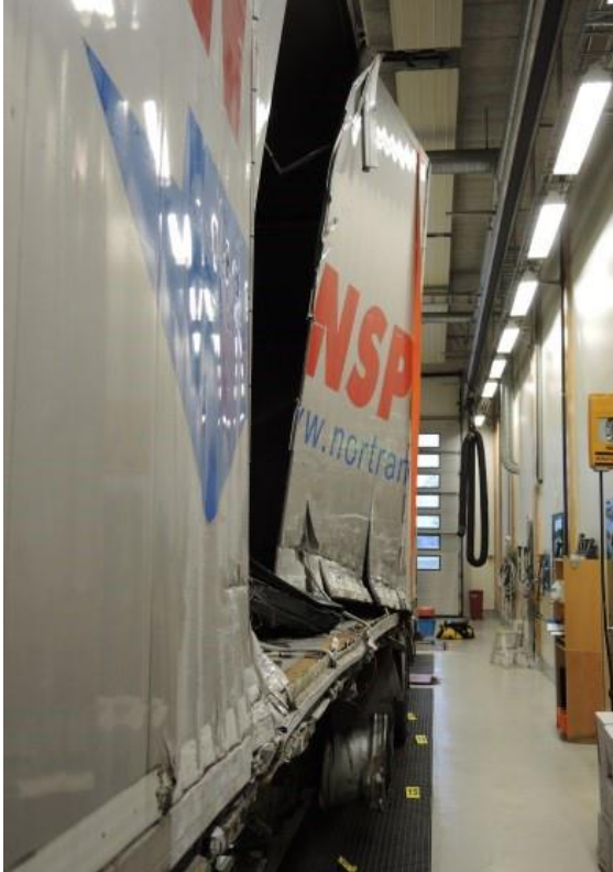
Figure 4: Damage to the left side of the semi-trailer. Photo: AIBN
