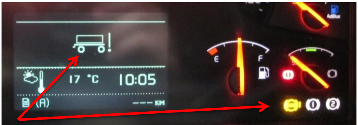
Figure 14: Dashboard display with ABS fuse for trailer installed. The EBS fault was now indicated on the dashboard. (The arrows show the lamps that would have been lit with the fuse installed.) Photo: AIBN
