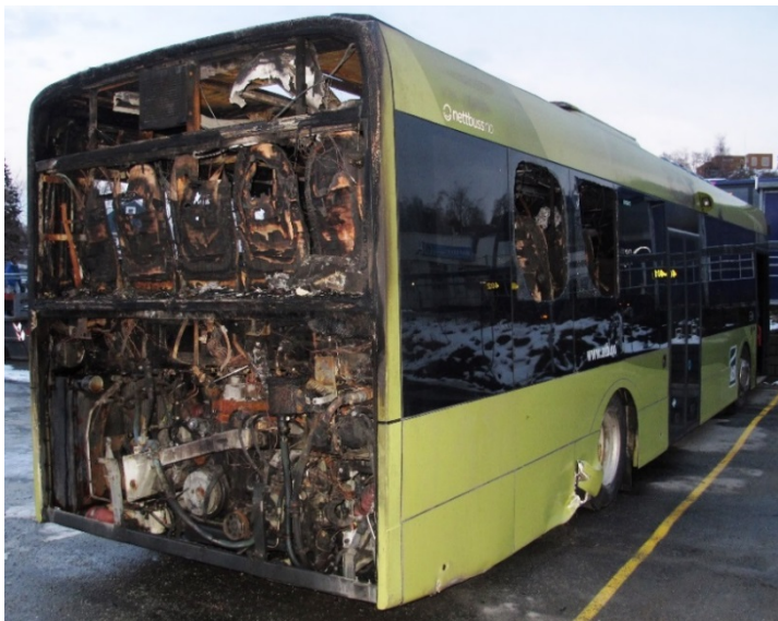
Figure 8: Fire on 13 November 2016. Damage to the engine compartment. Photo: AIBN
