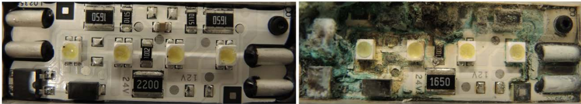
Figure 19: The interior of a new LED light shown on the left, and on the right a defective and corroded one. Photo: AIBN
