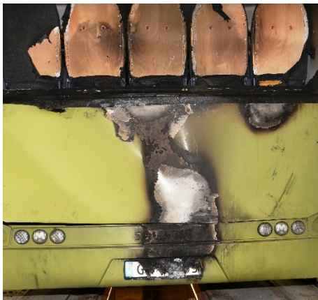
Figure 6: From the fire on 17 December 2016. Rear hatch placed in the position it was in before the fire. Photo: The police
