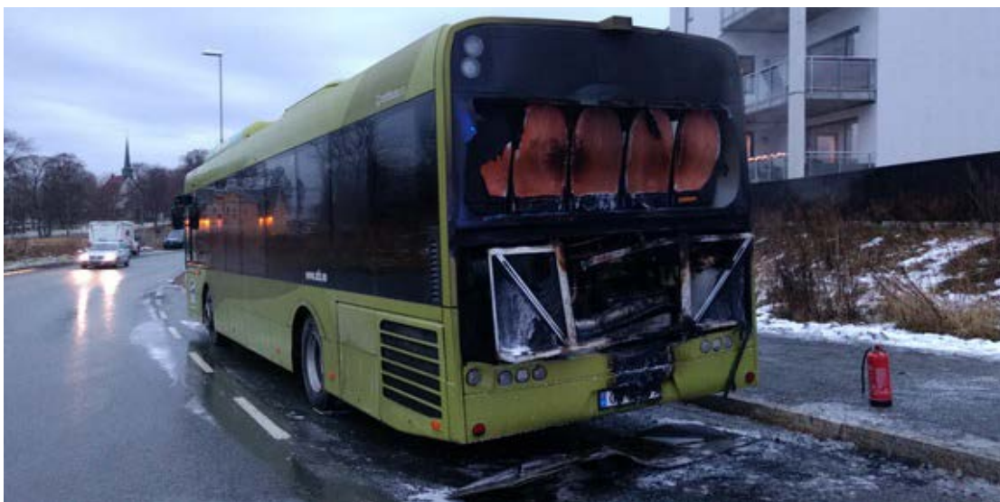
Figure 1: Fire damage to the rear of the bus, the engine compartment cover is lying on the ground behind the bus and the fire extinguisher is empty. Photo: The police
