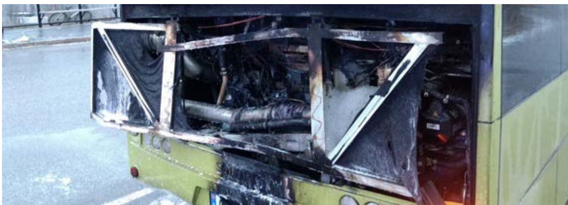
Figure 2: Close-up of the fire damage to the rear of the bus. Photo: The police
