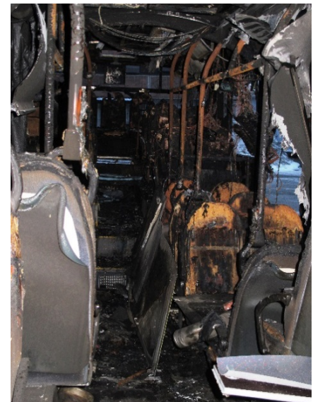
Figure 9: Fire on 13 November 2016. Fire damage to the interior, looking towards the rear of the bus. Photo: AIBN
