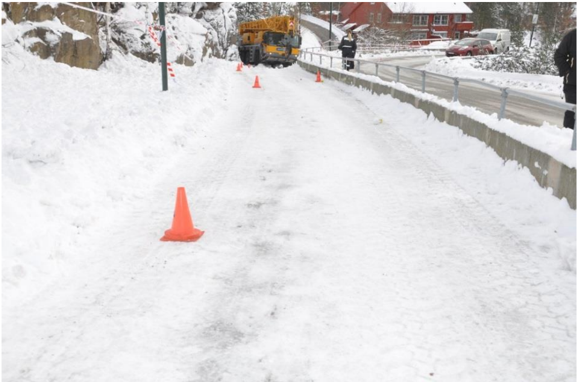
Figure 3: Tyre tracks and final position of the mobile crane. The first cone marks where the tyre track from the right front tyre changed character. Photo: The police
