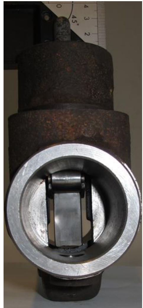
Figure 11: Assumed position of push rod and roller cage as shown in figure 5 and figure 6. Photo: AIBN
