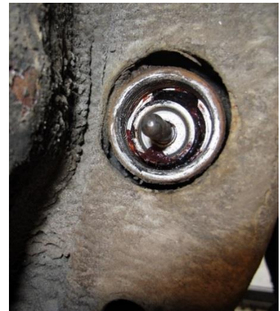
Figure 6: Push rod in expander assembly, wheel brake, left side. Photo: AIBN
