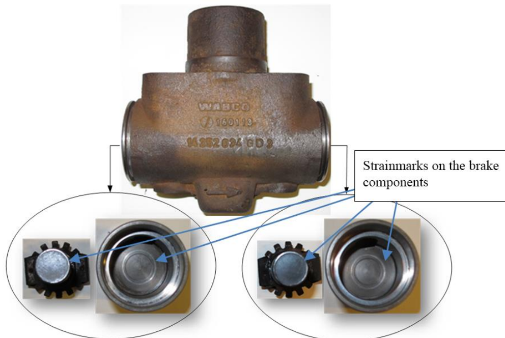
Figure 7: Physical traces of contact between the self-adjusting screw and the bottom of the wheel cylinder pistons on the left side, indicated by the blue arrows. Photo: AIBN
