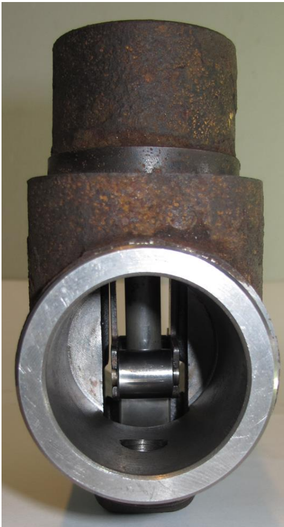
Figure 10: Roller cage 'slipped across'. Push rod with the wedge at the bottom of the housing and the roller cage at the transition between the wedge and push rod. Photo: AIBN
