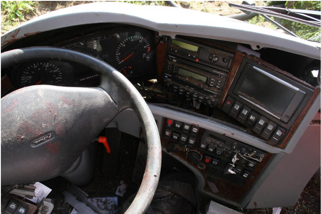
Figure 10: The driver's work station on the coach. The display on the right had GPS and a rear view camera. Photo: The police
