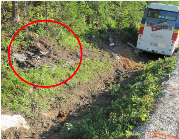
Figure 8: Road shoulder and ditch with the coach in its final position. Also shows the assumed initial location of the boulder that was pushed in front of the coach (red circle). Photo: AIBN
