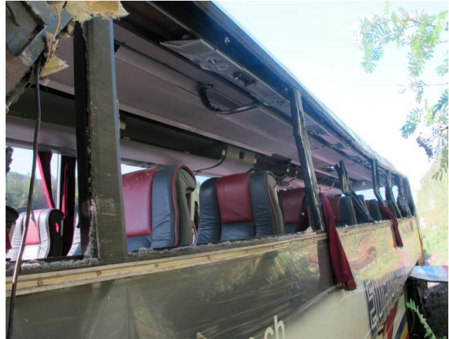
Figure 5: Damage along the left side of the coach. Photo: AIBN
