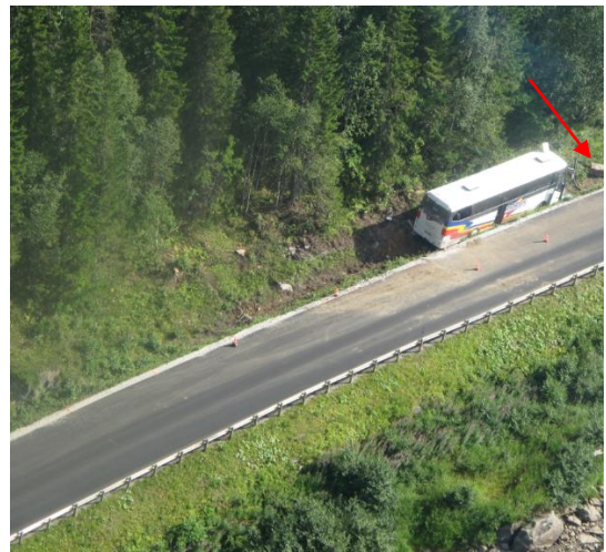
Figure 7: The accident site with the coach in its final position. The boulder that was pushed in front of the coach is just visible in front of the coach (red arrow). Photo: AIBN
