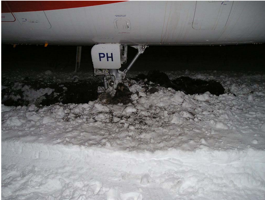
Figure 1. G-CRPH nose wheel sunk in the snow and soil.
