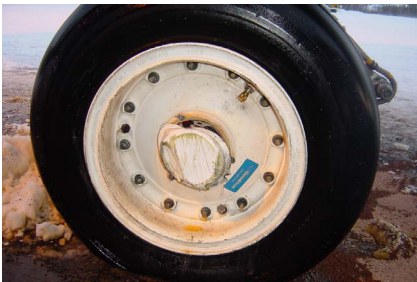
Figure 7. Left punctured nose wheel with damaged hubcap.
