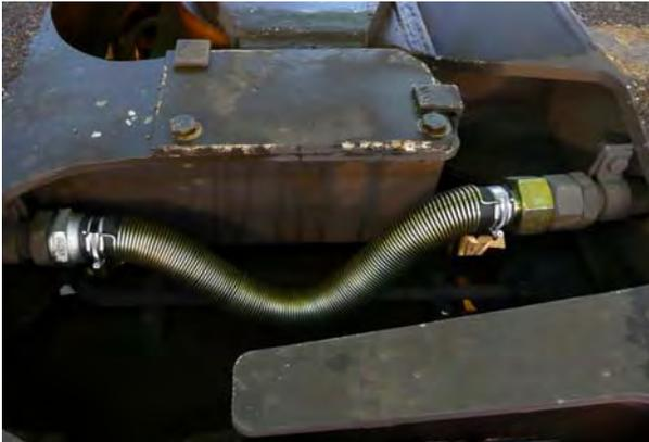
Figure 1: Brake hose above the middle bogie fitted without twisting.
