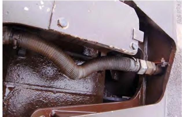
Figure 2: The brake hose on wagon 33684955117-9 was fitted with twisting.
