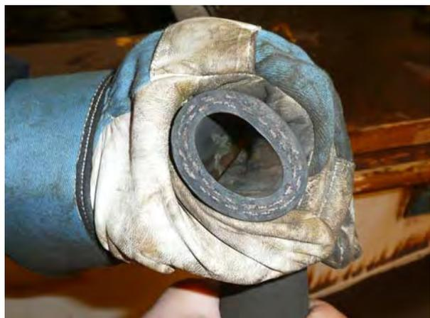
Figure 4: The cut brake hose could easily be squeezed together.
