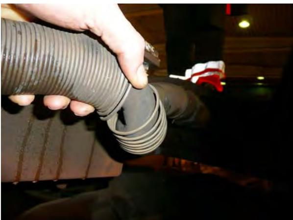
Figure 3: The twist in the brake hose resulted in a narrowing of the hose.
