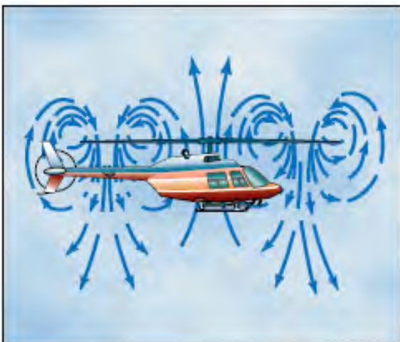
Figure 11-4. Vortex ring state.
