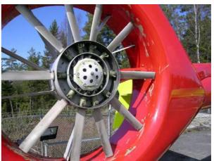
Fig. 4 Damaged tunnel and deformed blade tips
