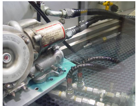
Figure 14: Fuel heater on the test bench.
