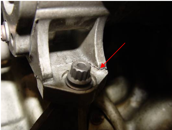
Figure 11: Fracture in the lower mounting lug on the fuel heater.
