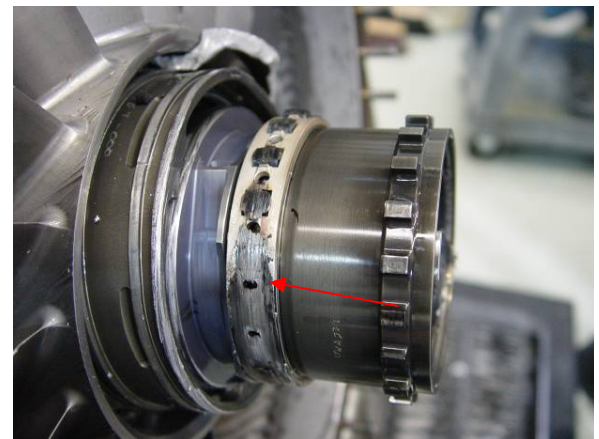
Figure 16: Bearing no. 2.5. The arrow is pointing at completely flattened rollers.
