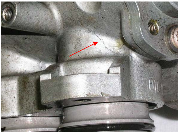
Figure 13: Crack going right through the fuel heater.
