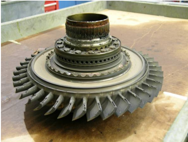
Figure 17: Carbon erosion on the first stage high pressure turbine (left engine).
