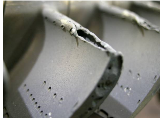
Figure 18: Close-up damage to turbine blade.
