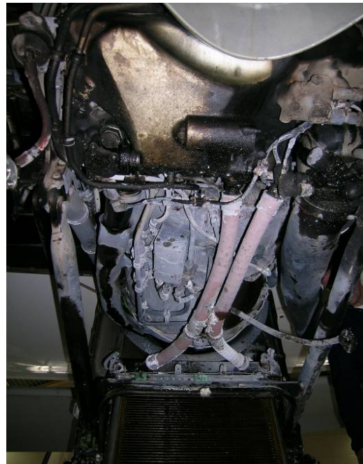
Figure 6: The underside of the engine viewed towards the back once the air intake section was lowered.
