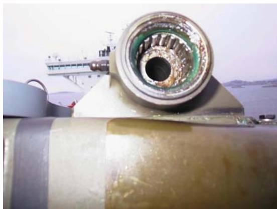
The remaining vibration absorber assy on Blue blade
