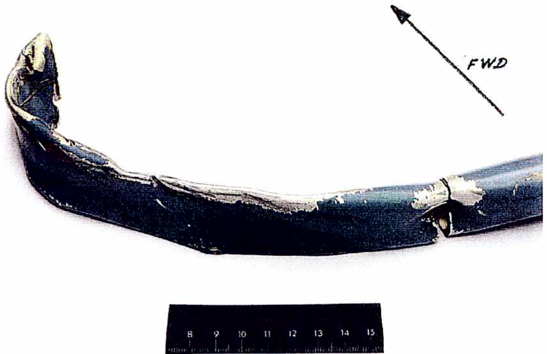
Fig. 11 Photo showing the two fracture locations of the TR pitch control rod, and the severely bent and flattened 22 cm rod section between the fractures. The forward direction of the helicopter related to the rod section is seen arrowed on the photo.
