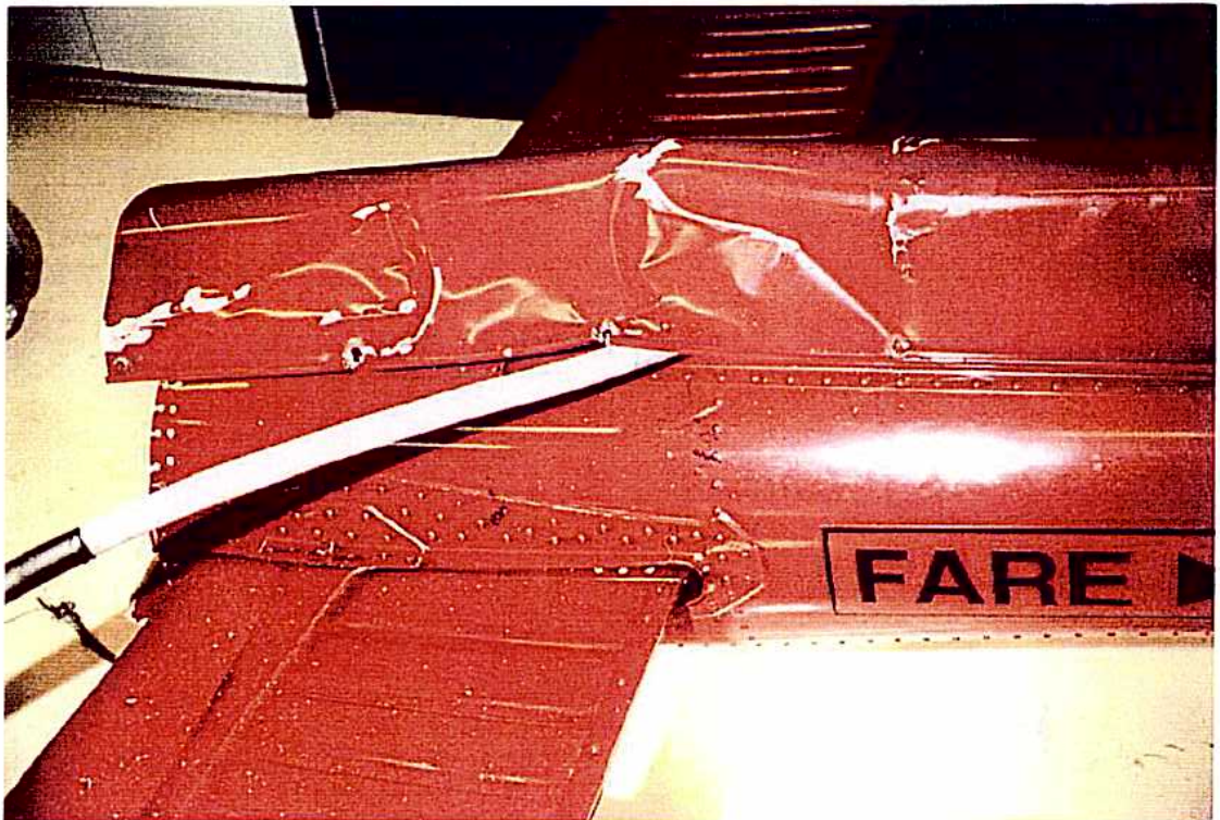
Fig. 5 Close-up photo illustrating bending and pulling of the TR pitch control rod through the fairing attachment, towards the L/H side of the helicopter. Photo by AAIB/N.
