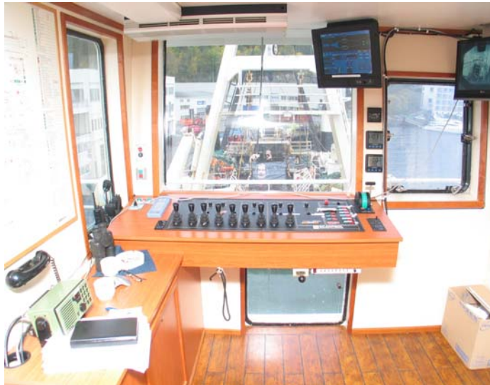
Figure 5: Operation panel aft in the wheelhouse.
