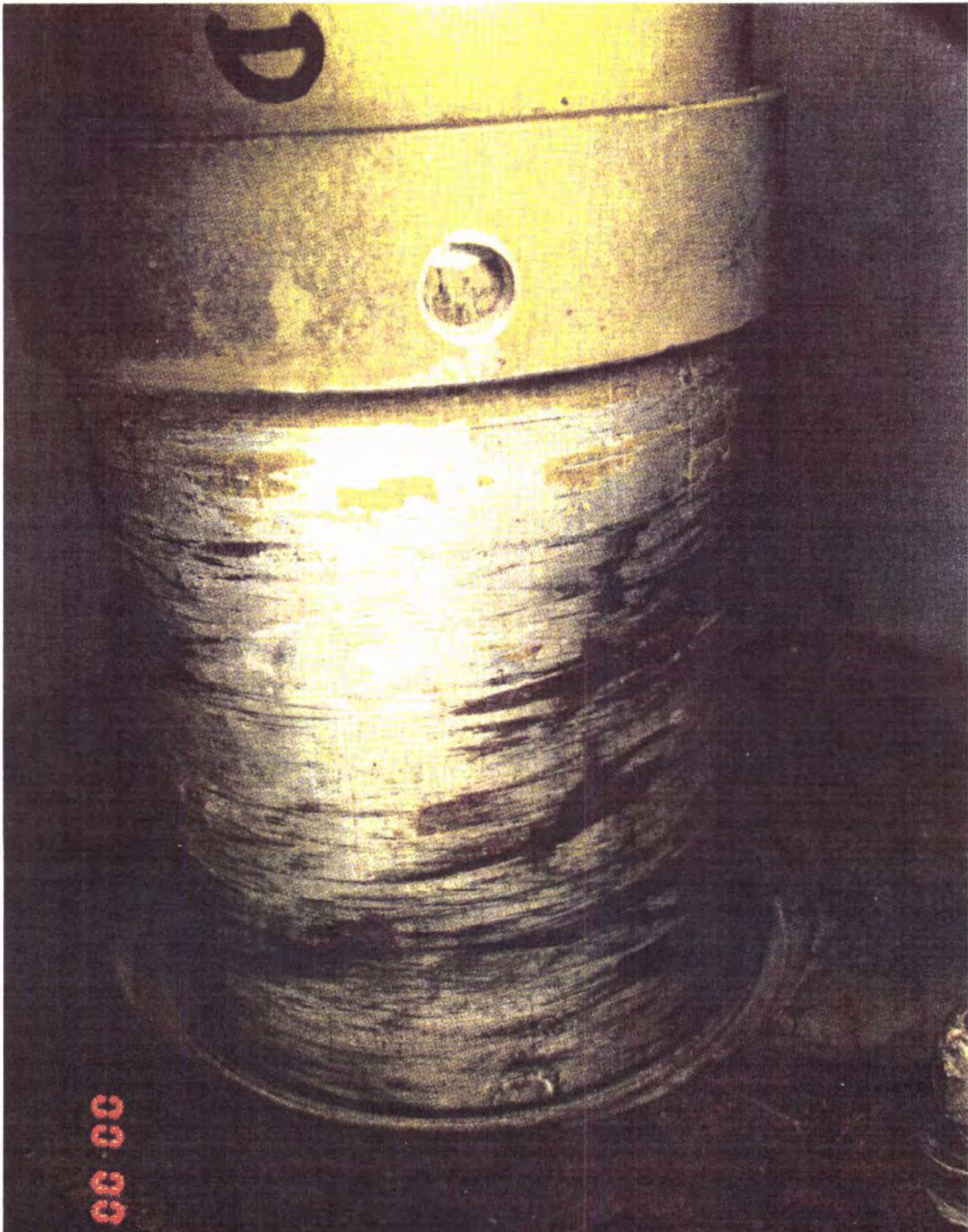
PHOTO 14 (FOTO) Clearly exhibits the extensive scoring. Note the circumferential length and angles of the score marks well in excess of the normal 35° of elevator travel. Some marks are up to 90° of the circumference.
