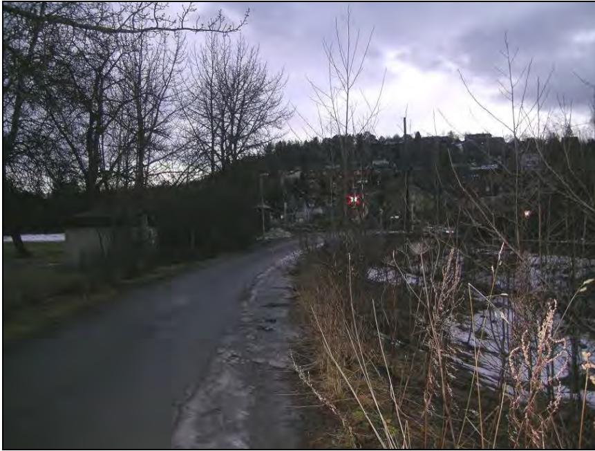
Figure 53 - Vegetation blocking sight lines to the level crossing (Stavne LC).
