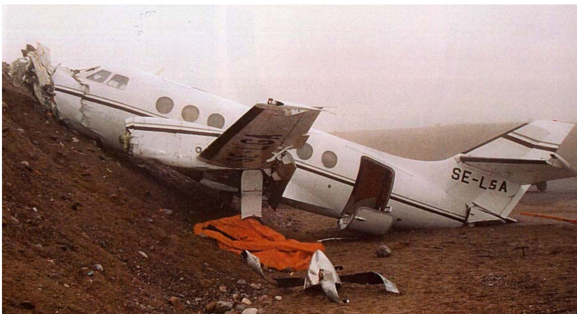
Photograph taken looking south the day after the accident. Note the unusual position of the wing, engine and landing gear
