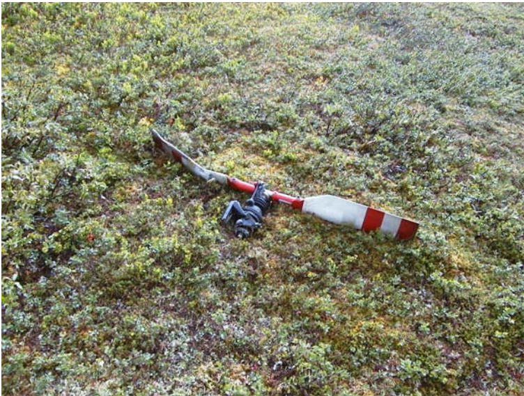
Fig. 2 SE-HSI Tail rotor with Output section of gearbox
