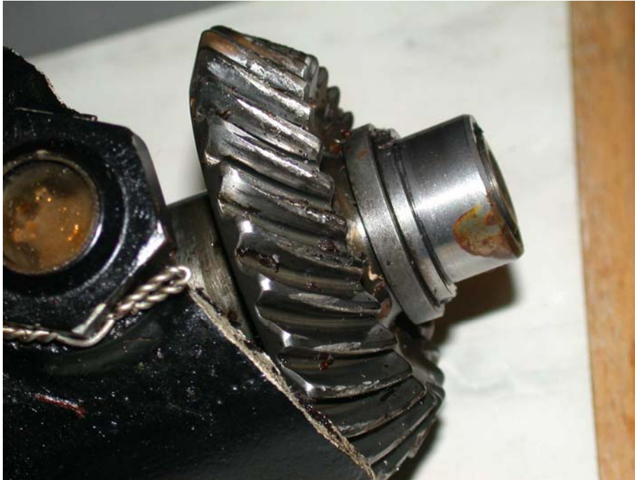
Figure 3 Photograph of output section gear. Examination using the stereo microscope concluded that the damage observed was secondary damage.
