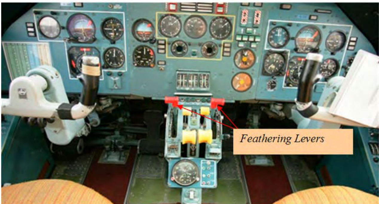
Figure 4: AN-28 Flight Deck with instrument panel, central console and red Feathering Levers.
